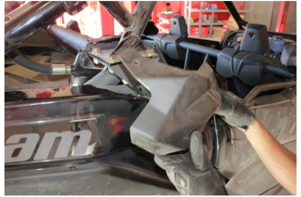
Step 20. Re-install the plastic cover fastened by 2 T30 screws.
