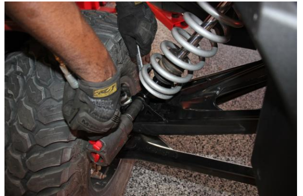
Step 17. Secure the coilover to the control arm with the OE hardware.
