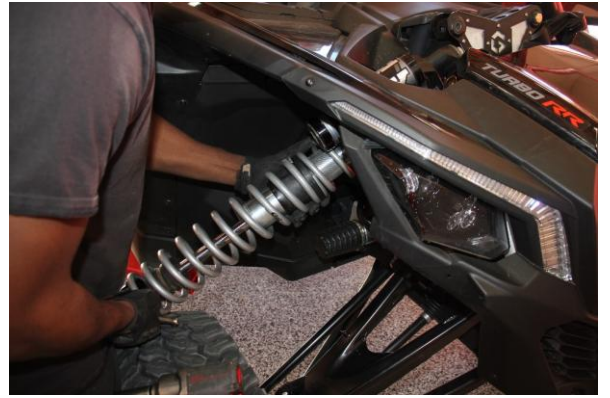
Step 14. Re-install the coilover.
