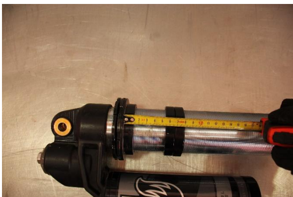
Step 9. Move the OE cross-over rings and set them at 80mm (3 9/64 IN) measuring from the spring flange to the bottom of the crossover rings.
