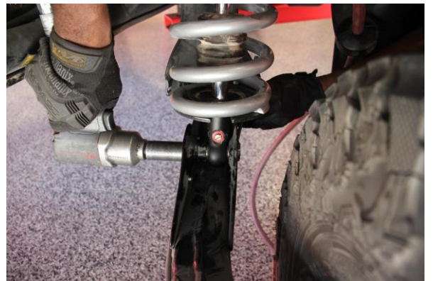
Step 18. Secure the coilover to the control arm with the OE hardware.
