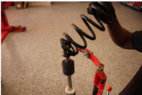
Step 7. Remove OE secondary spring.
