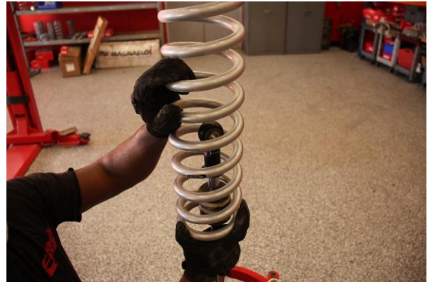
Step 14. Install the Eibach main spring.
