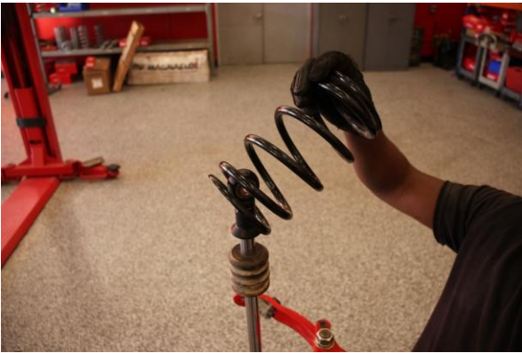
Step 9. Remove OE secondary spring.
