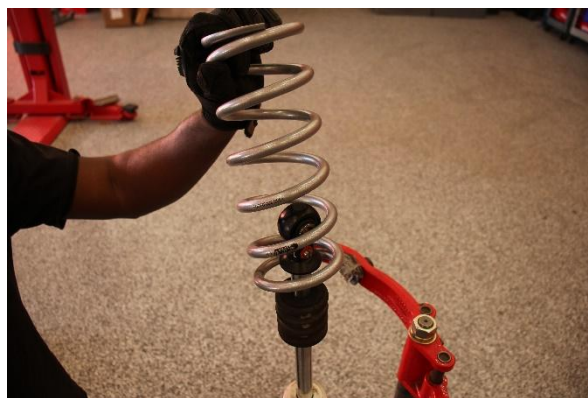
Step 10. Install the Eibach secondary spring.
