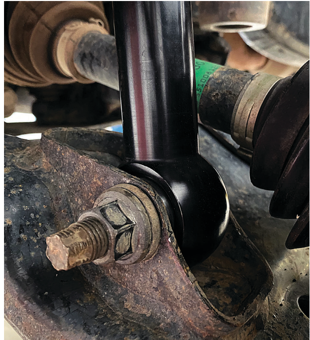
Fig. 4: Installed lower shock bolt.
