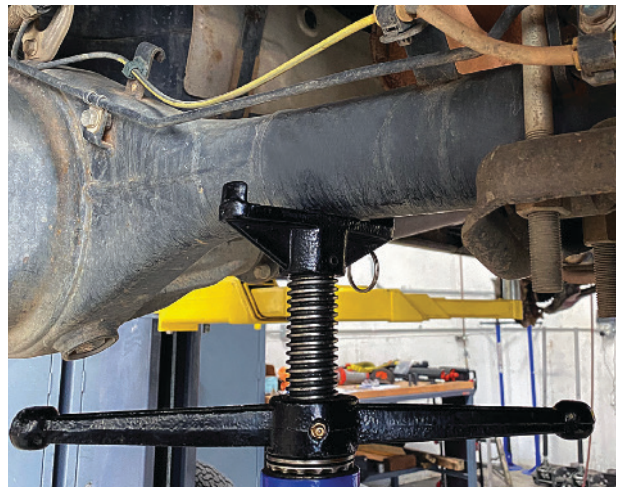
Fig. 12: Axle jack supporting the axle.
