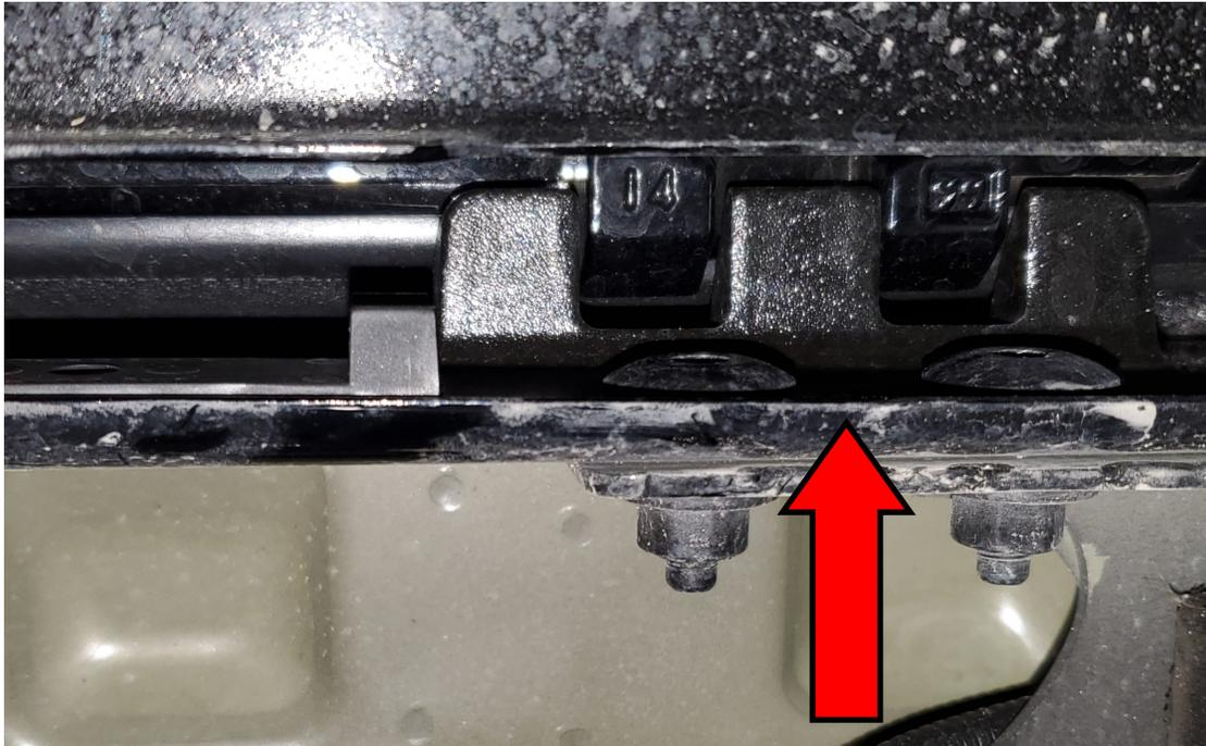
7. If your truck has a tailgate support and alignment bracket that interferes with the light bar installation, to get around this you can do one of the following:
