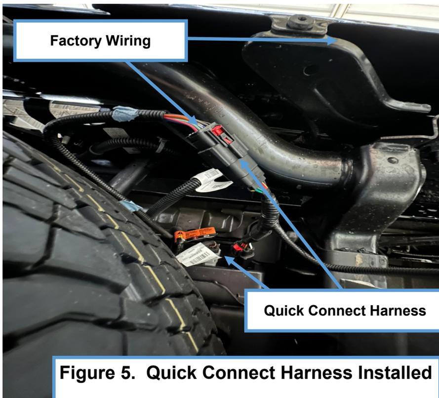
5. Route the Blade Quick Connect Harness along inner bumper and zip-tie safely into place.
