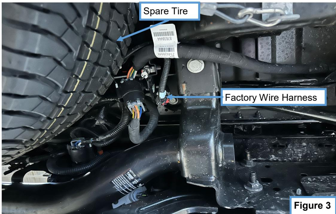
2. Disconnect the black plug shown in **Figure 3** (passenger's side pictured).
