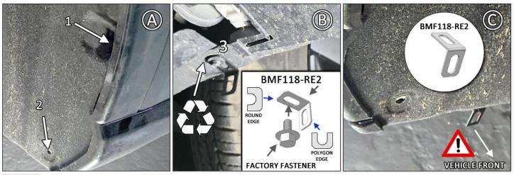
**IMAGE D** Place logo-side of flap facing rear bumper. Install SMWASH & HXBLT through flap & BMF118-RE2 mount 3. Fasten SMWASH & BLKNUT on logo-side mount 3.
