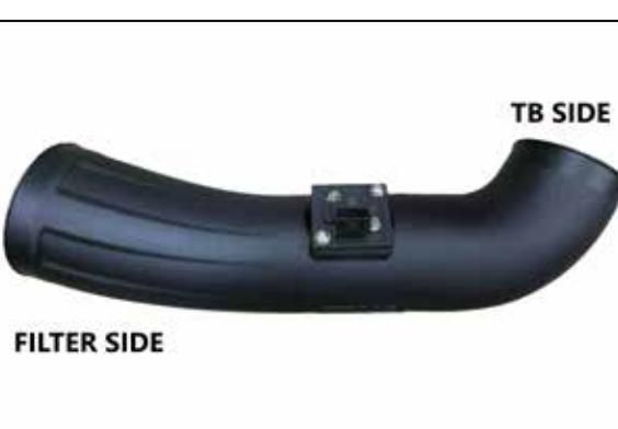
15. Install the MAF sensor assembly into the intake tube and secure using provided hardware. Secure and tighten. **NOTE: Make sure the sensor is going in the correct direction.**
