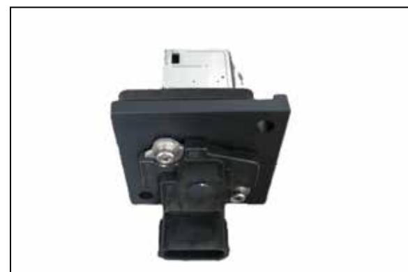
14. Install the mass air sensor into the provided adapter and secure with the provided hardware.
