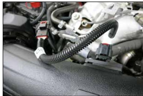
18. With provided MAF sensor harness extension, connect the original harness to the new harness and then to the sensor.
