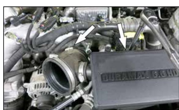
5. Loosen clamp on turbo housing, and loosen the nut holding in the resonator sound box and remove.
