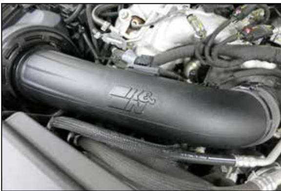
17. Install the intake tube assembly into the vehicle and position it into the K&N® filter and hump hose. Once positioned properly, tighten all clamps.
