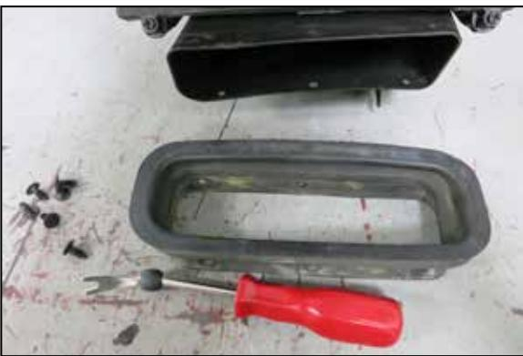
7. Remove the 6 push clips from the air box rubber hood seal on the stock air box. Remove the rubber hood seal. Save clips for next step.
