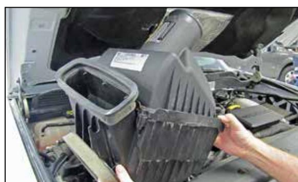
4. Lift up the air filter housing to release it from the mounting grommets and then remove the air filter housing from the vehicle.
