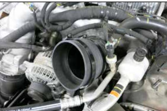
16. Install the hump hose with clamps to the turbo housing. Tighten the clamp on turbo housing only.
