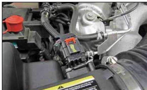
2. Slide the red locking tab back and then release the mass air sensor electrical connection.
