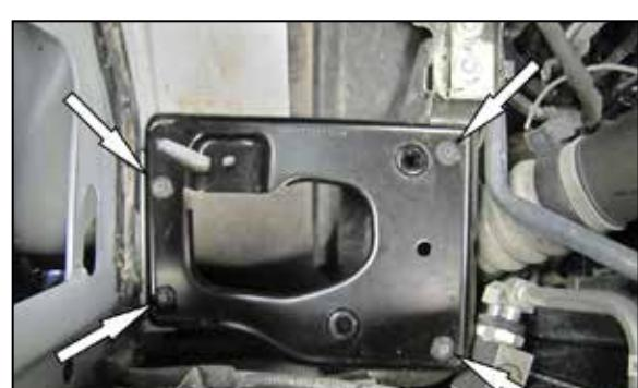
6. Remove the four bolts that secure air filter mounting tray and then remove the tray from the vehicle. Three of the factory bolts will be reused in a later step.
