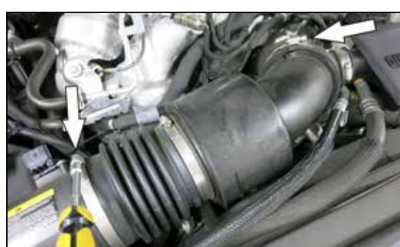
3. Loosen both clamps on the intake tube and remove.
