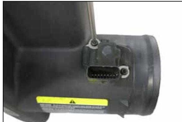
12. Remove the mass air sensor from the factory housing.
