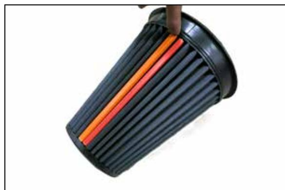
10. Attach the filter clips to the pleats on the air filter align and push down. Passenger side filters, place orange clip on top and red on bottom.
