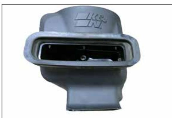
8. Install the factory rubber hood seal to the K&N® air filter housing. Secure using the 6 push clips.
