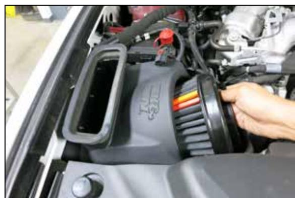
11. Install the K&N® air filter into the K&N® air filter housing.
