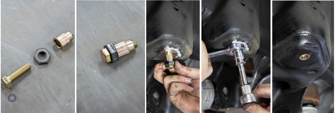
Figure 33: Install Tool for Rivet Nut
