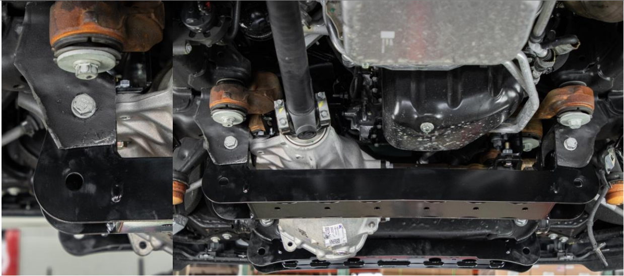
Figure 38: Install Rear Crossmember
