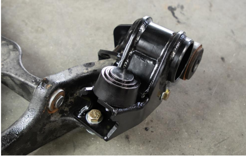
Figure 44: Install Outer Mounting Bolt and Bump Stop
