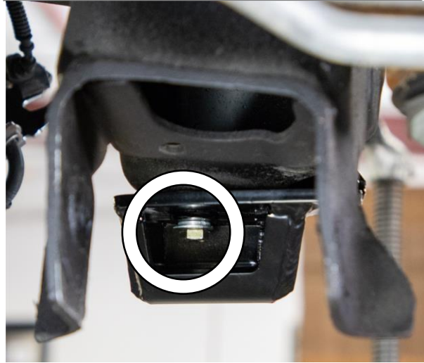
Figure 34: Bump Stop Installed
