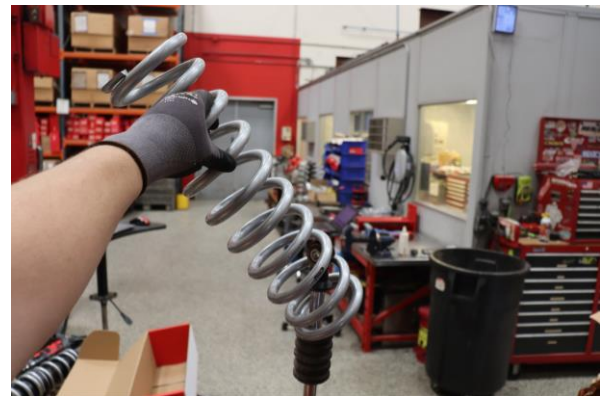
Step 18. Install the Eibach main spring.
