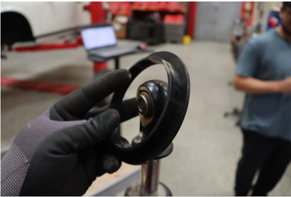
Step 15. Install the supplied Eibach spring adapter on the upper spring perch.
