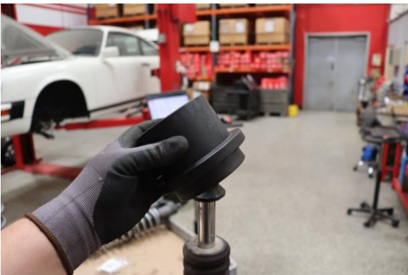
Step 17. Install the Eibach spring slider with the larger end facing away from the secondary spring.
