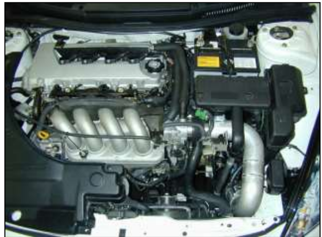
AEM ® intake system installed.
