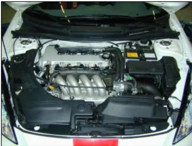
Stock air box system installed
