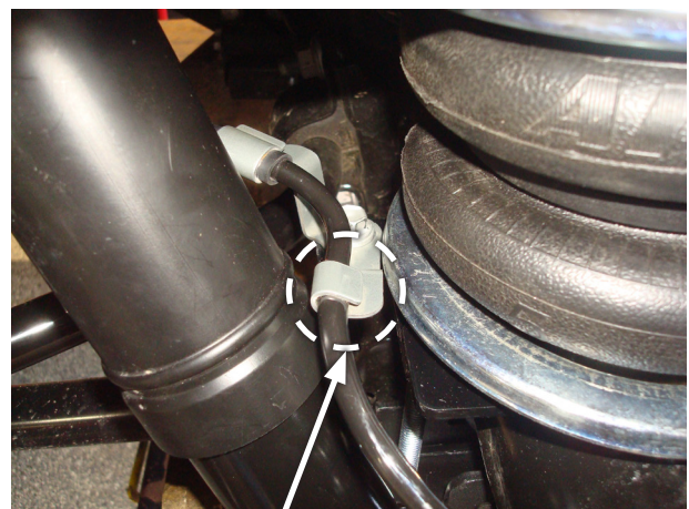
Adjust so there is clearance on both roll plate and shock before tightening hardware.
