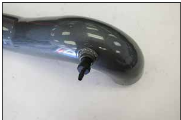
12. Install the 1/4" NPT vacuum fitting into the K&N intake tube as shown. NOTE: Plastic NPT fittings are easy to cross thread. Install the vent fitting "hand" tight, then turn it two complete turns with a wrench.
