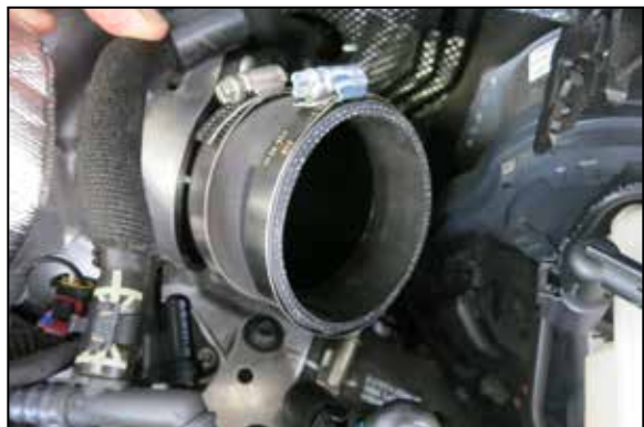
8. Install the provided step coupler onto the turbo inlet and secure with the provided hose clamp.
