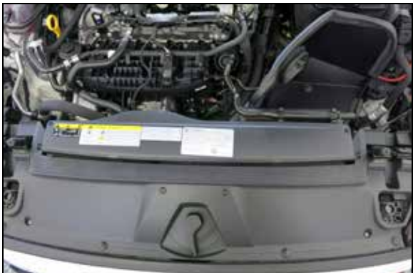
14. Reinstall the fresh air inlet and secure with the factory hardware.
