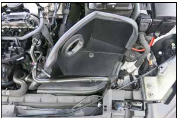
13. Set the heat shield into the vehicle so the mounting studs insert into the mounting grommets.
