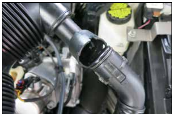
7. Depress the locking clips and disconnect the BOV hose from the intake tube and remove the intake tube from the vehicle.
