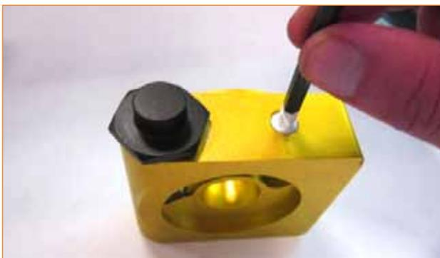
4. Wrench tighten the plug 2-3 full turns. (1/8" npt only)
