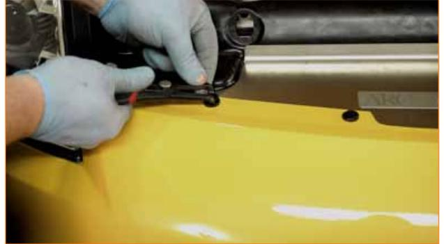
4. Remove the pop clips from the fender liner so you can access the remaining 10mm bolts that hold the bumper in place.
