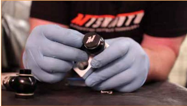
4. Place the sandwich plate onto the oil filter housing and secure it using the supplied M20 stainless steel adapter. Tighten this adapter using a 27mm socket.
