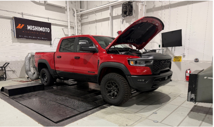
Figure 7: Mishimoto's 2025 Ram RHO loaded onto the MD-500XL-AWD chassis dyno. The vehicle must be run rear-wheel-drive as it is too long to fit on the dyno.
