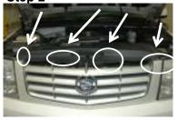
Remove push pins located on top of the grill
