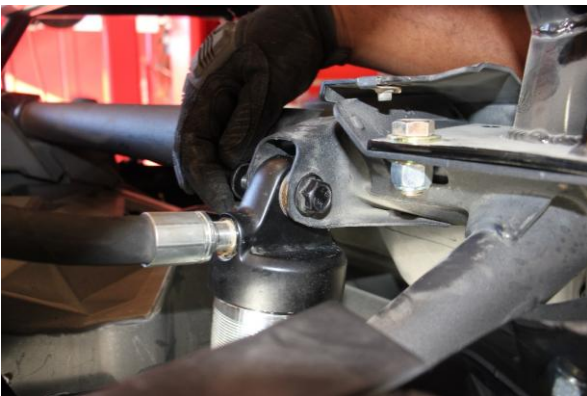
Step 17. Secure the coilover to the upper mount with the OE hardware.
