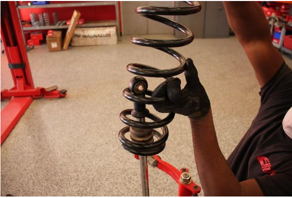
Step 7. Remove OE main spring.
