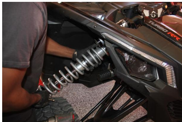
Step 14. Re-install the coilover.
