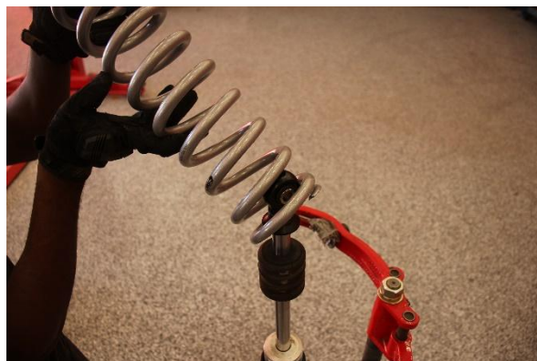
Step 12. Install the Eibach main spring.
