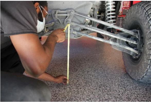
Step 21. Measure from the ground to the center of the lower radius arm bolt. The recommended preload measurement in Step 10 will get the vehicle close to the recommended ride height but each vehicle may vary some. As reference, skid plate measurement at recommended preload should be 406.4 mm (16 in.). We recommend setting the ride height at 490mm (19 19/64in.) measuring from the ground to the center of the lower radius arm bolt. Note: If you have larger than stock wheels and tires, the ride height will be increased. Due to the sensitivity of weight of these vehicles, weight distribution may change ride heights, additional pre-load may need to be added to compensate.
