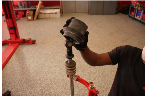
Step 8. Remove OE slider.
