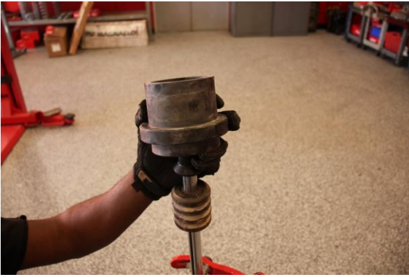
Step 13. Install the OE spring slider.
