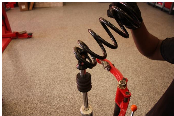
Step 7. Remove OE secondary spring.
