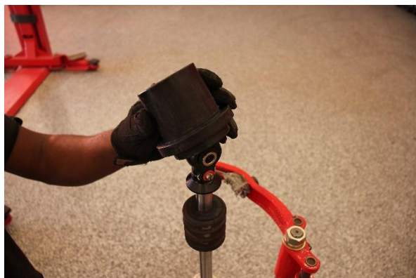
Step 11. Install the OE slider.
