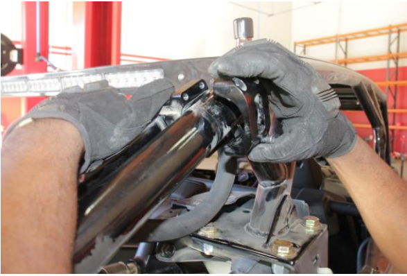
Step 19. Re-install the resi mounting bracket, secured by the 4 socket head cap screws.
