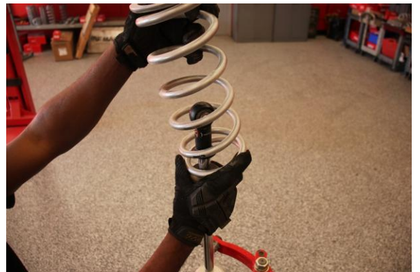
Step 12. Install the Eibach secondary spring.
