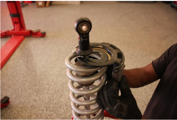
Step 15. Compress the spring assembly and re-install the spring retainer.
