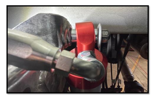
12. Using an 18mm socket and 21mm wrench, install the lower shock bolt and nut with the included misalignment spacers as shown in the below photo. You may need to raise or lower the axle slightly to align the bolt with the eyelet. Torque the bolt and nut to the factory specification shown in the table on the last page.
