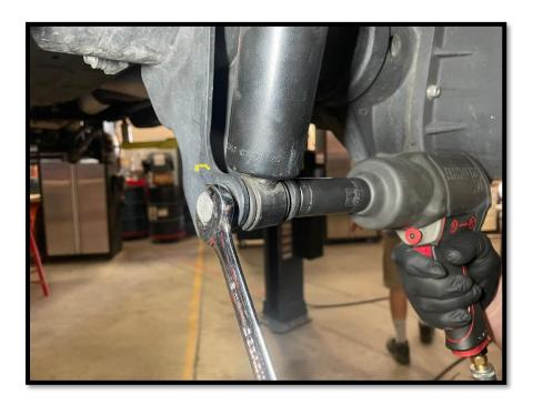
6. Using an **18mm** socket, remove the upper shock nut.
