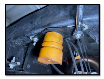
9. Using a **15mm** socket, install the reservoir bracket on the factory frame studs, between the bump stop and the frame rail, as shown in the below photo. Torque the bump stop mounting nuts to the factory specification shown in the table on the last page.
