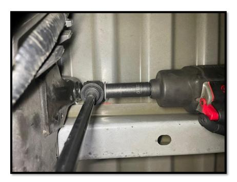
7. Using a prybar, remove the upper shock bushing from the frame mounting stud, and remove the shock completely.
