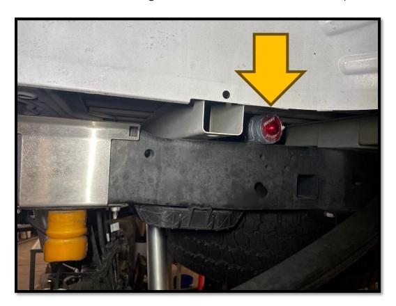
11. Using an **18mm** socket, install the upper shock nut with the included frame stud spacers on each side of the top cap bearing as shown in the below photo. Torque the nut to the factory specification shown in the table on the last page.
