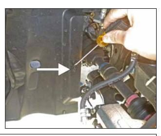
d. Undo the harness clip attached to the back side of the plastic cover.
