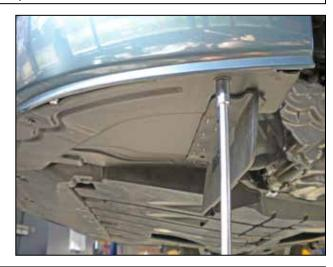
f. Remove the three 8mm bolts/screws along the outer edge of the front portion of the wheel liner on the driver side.
