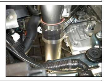
g. Use the 2.75"x3" coupler to attach the lower pipe to the upper pipe, using the supplied (#9448) hose clamps. Fasten the intake pipe bracket to the threaded soft mount with the supplied nut and bolt.
