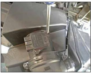
c. Remove the MAF sensor from the stock airbox assembly.
