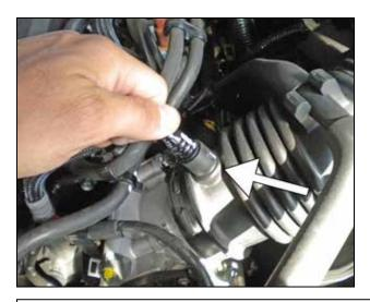
g. Pull out the PCV hard line from the nipple located just in front of the throttle body.
