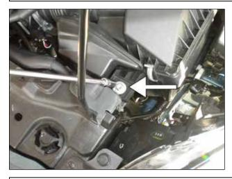
k. Remove the 10mm bolt securing the airbox to the core support.
