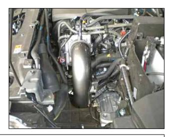
e. Install the upper intake pipe into the coupler installed earlier in step 3b. Reattach the MAF harness connector to the MAF sensor.
