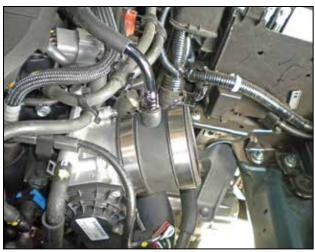
b. Install the coupler with the nipple onto the throttle body using the provided hose clamps (#9448).
