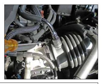
h. Loosen the 10mm hose clamp so that the rubber boot can be removed from the throttle body.
