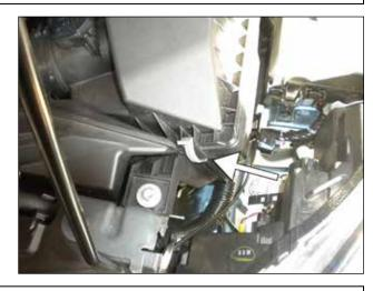
I. Unlatch the 2 metal retaining clips securing the air box lid.
