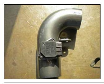
d. Install the MAF sensor into the upper intake pipe using the supplied bolts.
