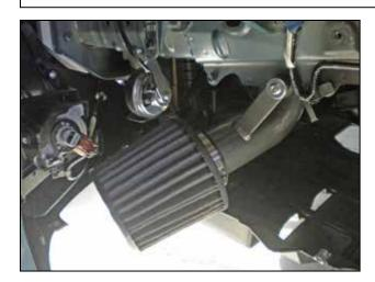
h. Attach the AEM® air filter onto the lower intake pipe. Once proper fitment is acheived, secure the air filter to the intake pipe with the provided hose clamp (# 9444).
