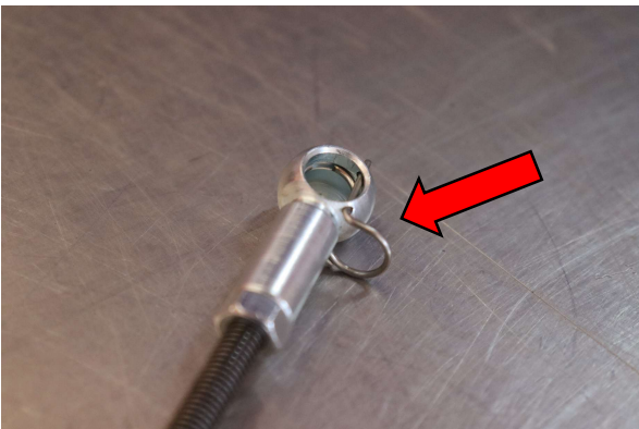
Remove secondary clip from socket before install.
