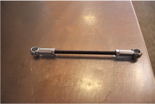
Aftermarket ride height sensor rod required for any RHO that is lifted 2 inches and above.
