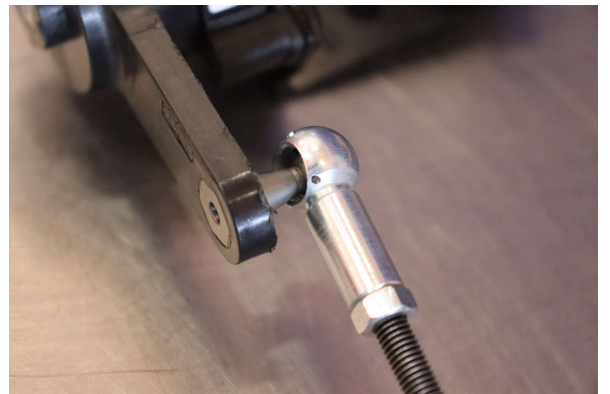
Install new ride height sensor rods on the front. Firmly press socket onto sensor and upper control arm. This rod allows frame mounted sensors to be at factory angle for proper operations on the active terrain dynamics system.
