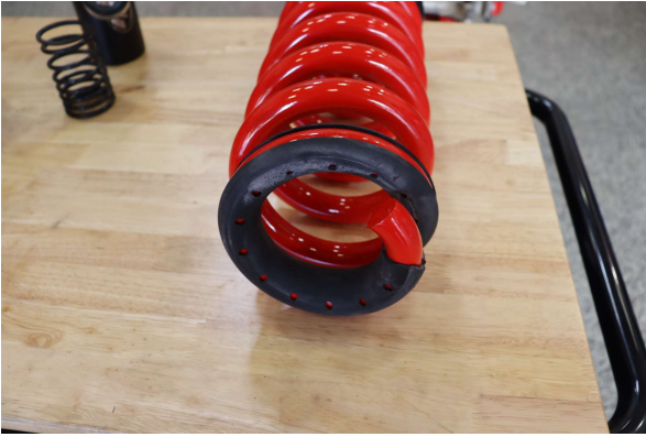
The bottom piece of tubing from the OE springs on the front and rear must be removed and installed on the Eibach springs.
