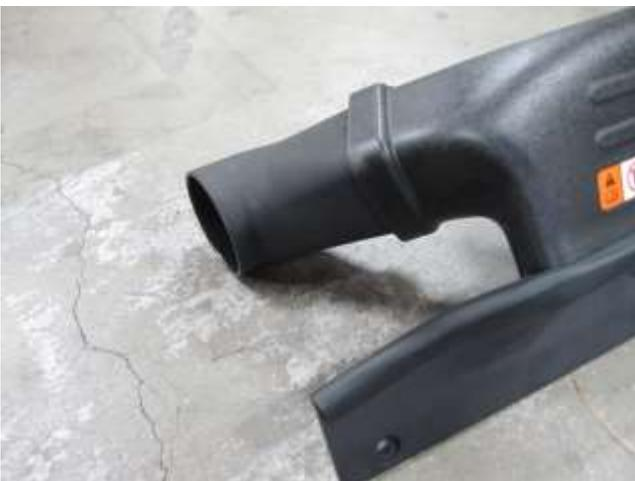
o. Place the adapter scoop into the stock scoop.
