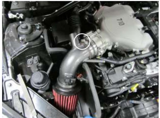
j. Install the AEM intake tube into the coupler and tighten the other hose clamp.
