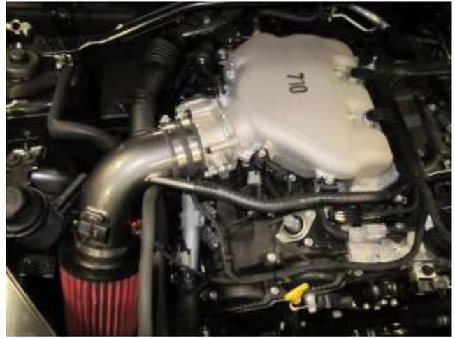
l. Slide the vent tube onto the AEM intake and secure with the stock spring clamp.
