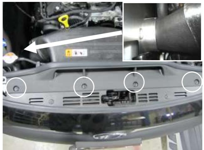
p. Install the scoop into the vehicle aligning the scoop adapter into the hole in the heat shield. Reinstall the engine cover.
