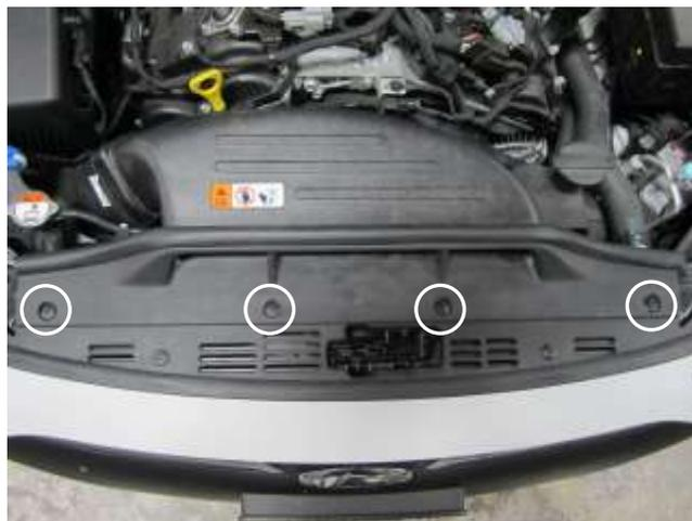
b. Remove the 4 plastic screws that hold down the air scoop. Note: These will be reinstalled in step 3p.
