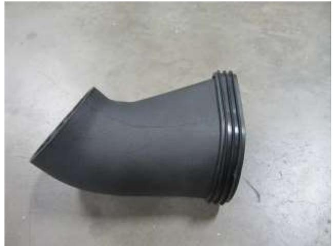
n. Install the seal onto the adapter scoop (9-0437) that was removed in step 2i.
