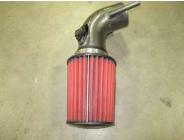
i. Install hose clamp (9456) and AEM filter onto the intake tube. Tighten clamp.
