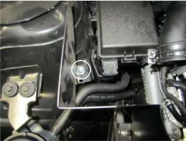
e. Align the heat shield with the mounting location shown and install the bolt (22224), and two washers (1-3025 & 08275) to the vehicle.
