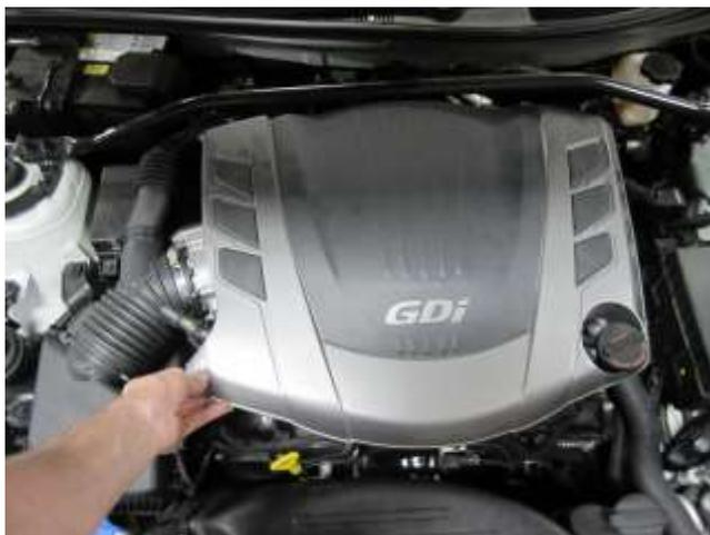
a. Pull up on the engine cover and remove it.
