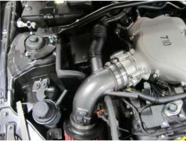
k. Slide the sound tube onto the AEM intake and secure with the stock clamp.
