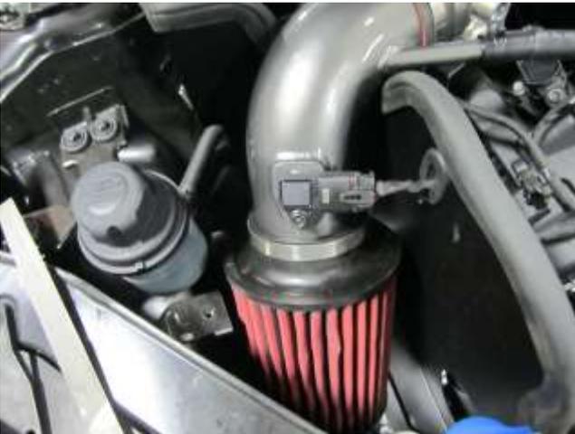
m. Connect the temperature sensor connector to the sensor.
