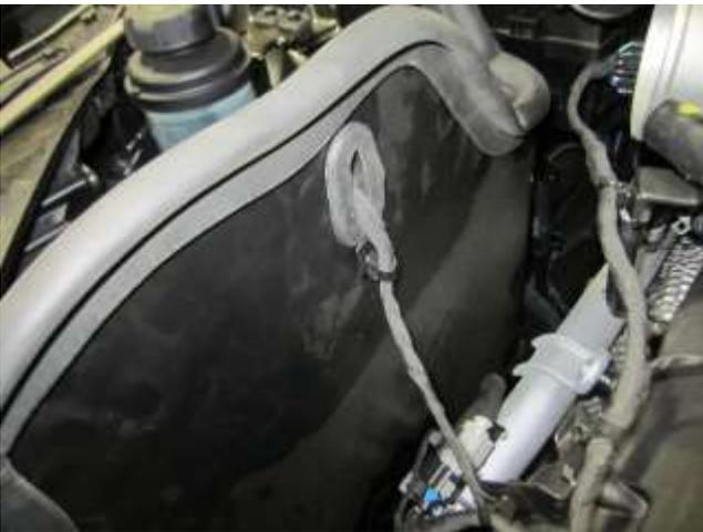
g. Slide the temp. sensor connector through the grommet (784640) and heat shield, then squeeze the grommet and install into the heat shield as shown.
