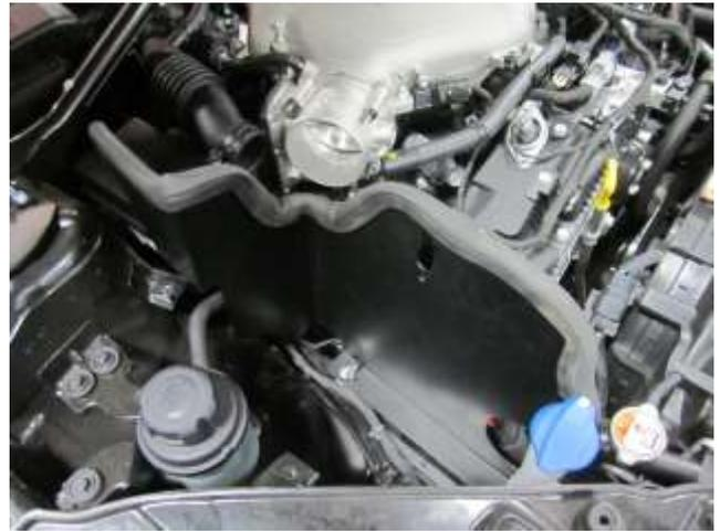
f. Install the edge trim (102496) onto the heat shield at this time.
