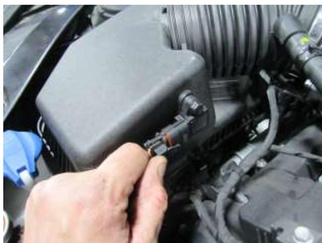
c. Unplug the intake temperature sensor by depressing the clip and pulling away from sensor.
