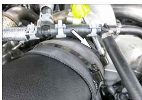
14. Slide the coupler onto the turbo inlet, adjust the assembly for best fit, then tighten the clamps on inlet coupler.
