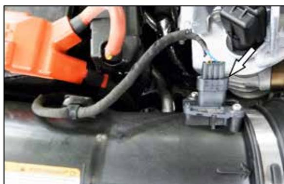
2. Disconnect the mass air sensor electrical connection and unhook the wiring harness from the air filter housing.
