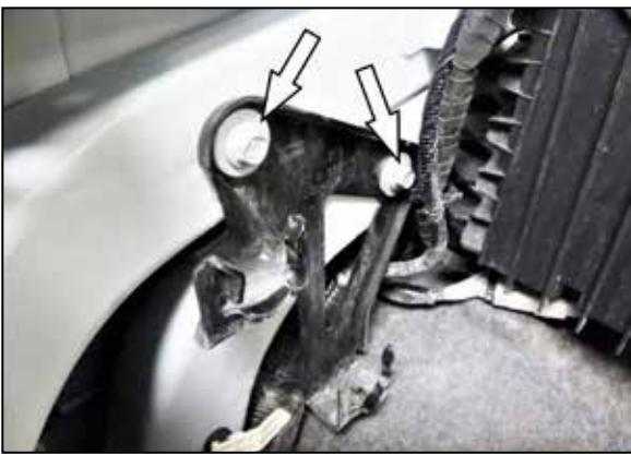
7. Remove the two bolts securing the air filter housing bracket to the inner fender, then remove the bracket from the vehicle.
