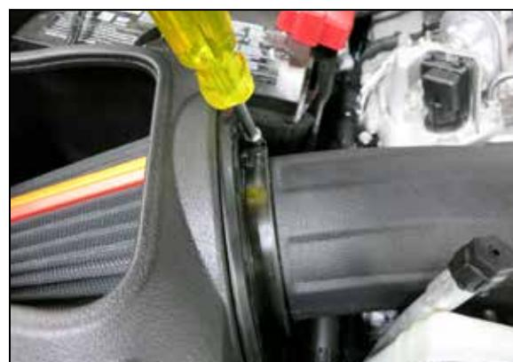
13. Install the K&N intake tube into the air filter and align with the turbo inlet. Make sure the bead on tube is locked into filter and tighten filter clamp. **NOTE: Filter base can rotate in housing, allowing the tube to sit properly in hump hose on the turbo.**
