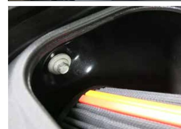
9. Install the K&N air filter partially into the K&N air filter housing. Install the housing and filter assembly into the vehicle, then secure the housing to the inner fender with one of the bolts from step #7. Do not tighten bolt yet.
