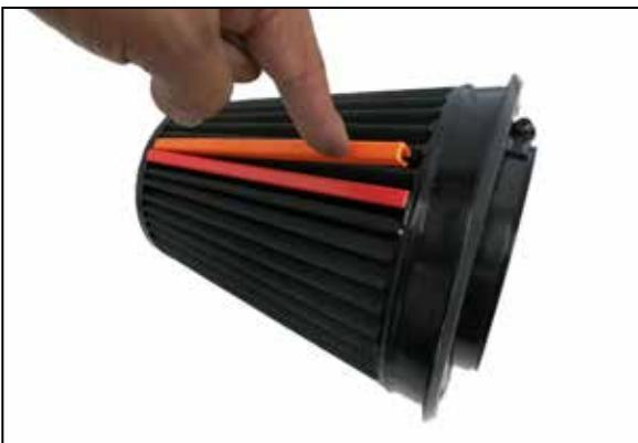
8. Attach the filter clips to the pleats on the air filter, align them and push down. Passenger side filters, place orange clip on top and red on bottom.
