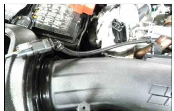
16. Using the provided extension harness, reconnect the mass air sensor electrical connection.
