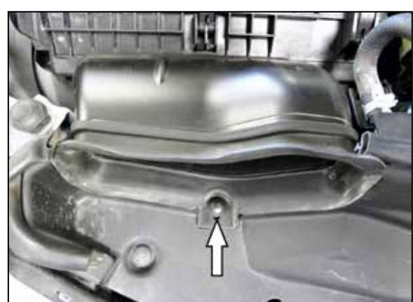
5. Remove the pin that secures the fresh air intake duct, then remove the duct from the vehicle.
