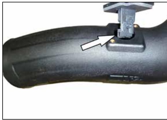
11. Install the mass air sensor assembly into the K&N intake tube so that the opening of the sensor is towards the filter end of the tube. **NOTE: Make sure the sensor is going in the correct direction.** If it is not installed in the correct orientation, remove the adapter bolts and spin 180 degrees then reinstall the bolts.
