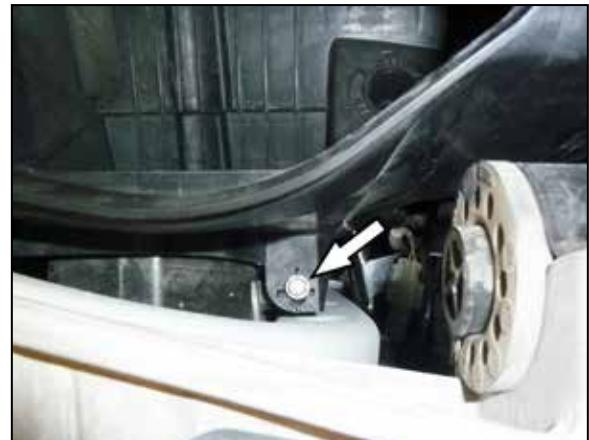
6. Remove the bolt securing the air filter housing, then remove the housing from the vehicle.
