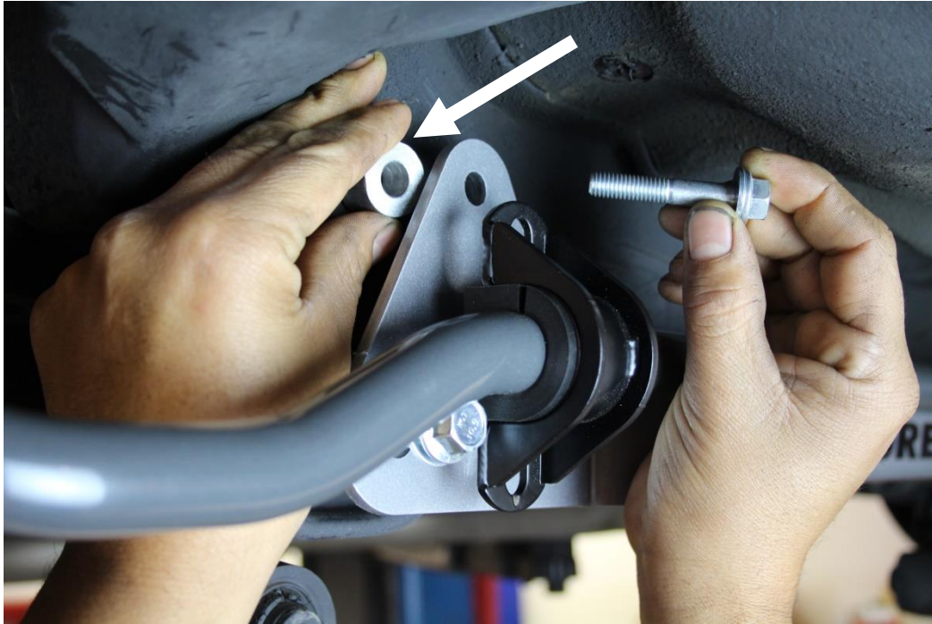
Use the short spacer between the brace and chassis (c)
