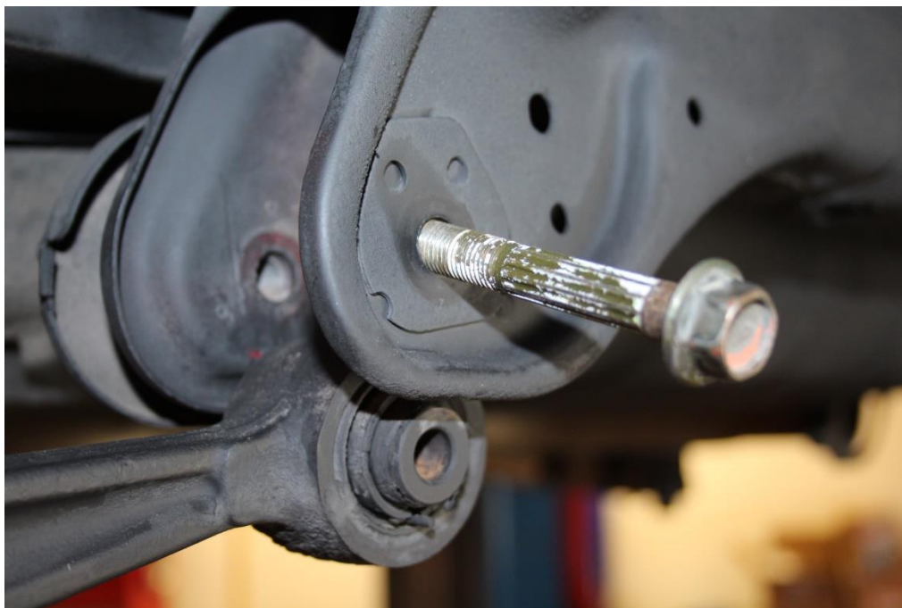
Remove the lower control arm bolt. (a)
