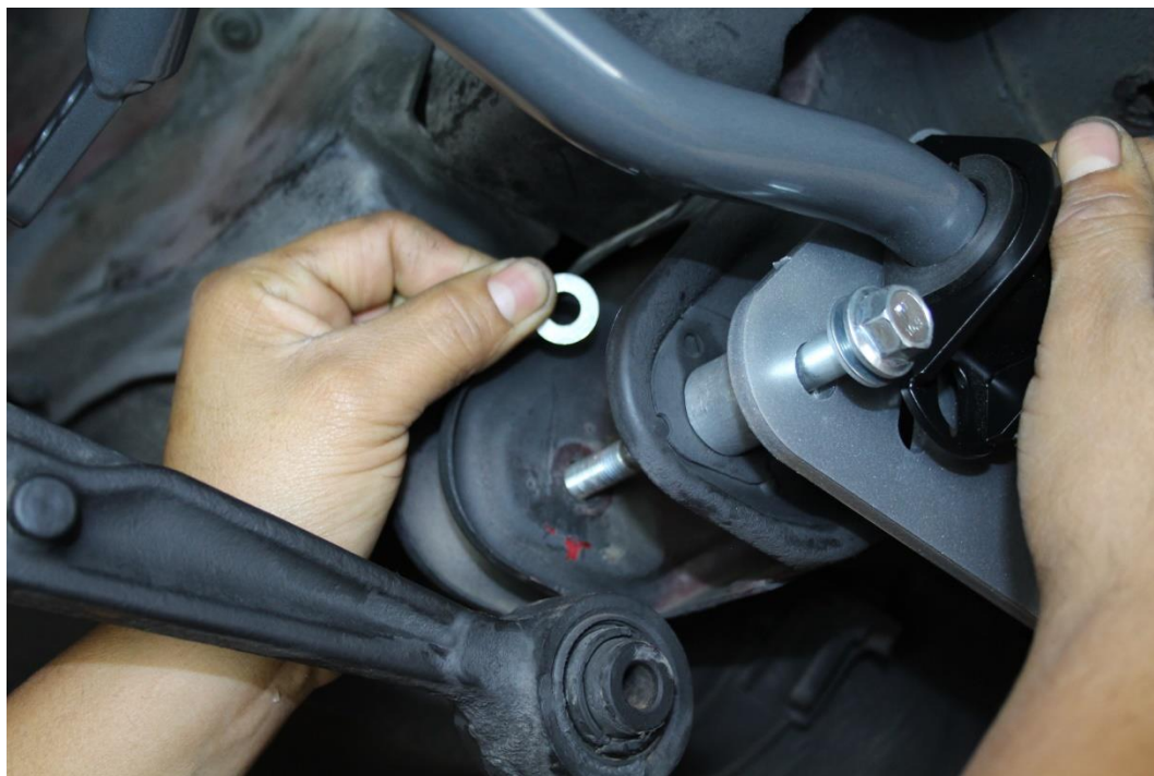
Use the nylock nuts and washers to secure the upper mount if not equipped with factory mounting holes (d)
