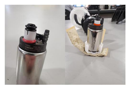
6 – Install the pump into the center section, all 3 of the O-rings should be seated inside the inlet of the module center section, lock the pump into place by latching the three lock tabs on the filter sock retainer.
