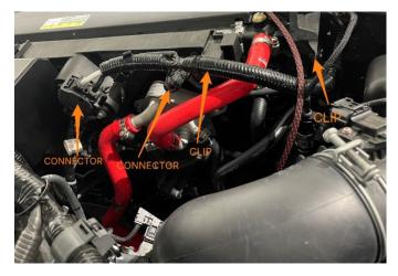
**16.** Disconnect the small upper radiator hose from the radiator and the second coolant hose connected to the transmission cooler. (See image on the right)
