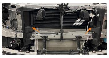
**30.** Take the Mishimoto rubber duct and line it up with the 2x holes in the side ducts and the hole in the black middle bracket, then place the included flat bracket underneath the duct and thread in the included 4x 8mm bolts into the threaded holes on the bottom of the intercooler. Tighten each bolt hand tight and then tighten each bolt to approx. 50 in-lbs. Check to make sure that none of the bolts have become loose during this process as the rubber depresses causing the bolt to come loose.
