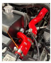
**14.** Remove the 2x 10mm coolant reservoir bolts that secure the reservoir to the fan shroud. As you remove the coolant reservoir, there will be one hose connected to the bottom of the reservoir, remove this hose from the reservoir and remove the reservoir from the vehicle.
