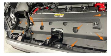
5. Remove the 3x 10mm bumper bolts at the top of the bumper. Then, disconnect the 2x electrical connectors on the passenger side of the bumper. Vehicles with a front bumper camera will also have another electrical connector on the driver's side of the bumper which also must be disconnected.
