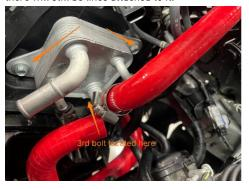
**18.** Clamp off the two transmission lines connected to the radiator and then remove the lines from the radiator. Be careful to clean up any transmission fluid that comes out. It is helpful to cap off the fittings on the radiator to prevent leakage during removal.
