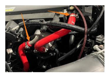
17. Remove the 3x 10mm bolts securing the transmission cooler to the fan shroud. Set the cooler aside but do not completely remove it, as there will still be lines attached to it.
