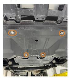
3. Place a bucket underneath the driver's side of the radiator and begin draining the coolant from the radiator by loosening the drain valve. Once the coolant starts to flow, remove the coolant reservoir cap from the reservoir to allow the coolant to flow freely. (Mishimoto Reservoir shown). The drain valve will be slightly higher on the radiator end tank on the hybrid models.
