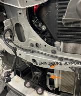
**29.** Reinstall the 2X side ducts on the core support and install the 3x (6x total) push clips on each side.
