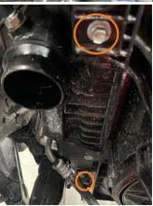
23. Remove the 4x (2x bolts and 2x nuts) 10mm fasteners holding the A/C condenser to the radiator. In addition, remove the 1x 10mm bolt holding the A/C line to the core support to allow more movement in the A/C condenser. Carefully remove the A/C condenser from the radiator and let it sit on the lower core support or use bungee cords to support the A/C condenser during radiator removal.
