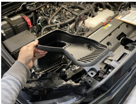
2. Remove factory air scoop.
