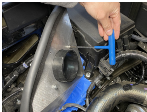
15. Bolt velocity stack to heat shield using the (4) provided 12mm hex bolts through intake tube side of heat shield.
