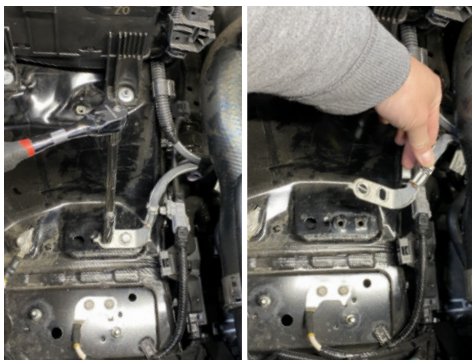
10. Using a 12mm socket, loosen and remove bolts to disconnect the chassis ground. Save bolts for use later.
