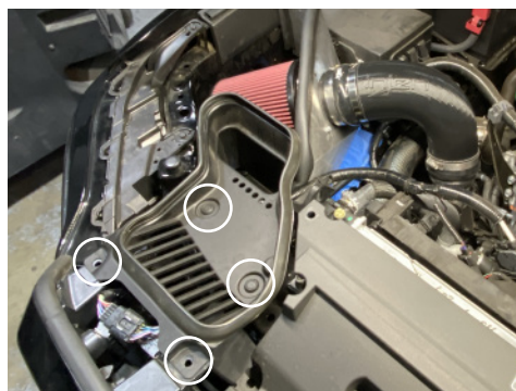
24. Secure using factory push pins.
