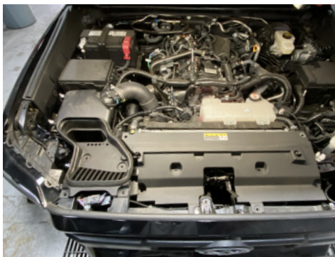
1. Factory intake system.
