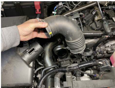
5. Loosen clamps and remove factory intake tube.
