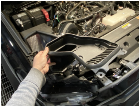
23. Reinstall factory air scoop.
