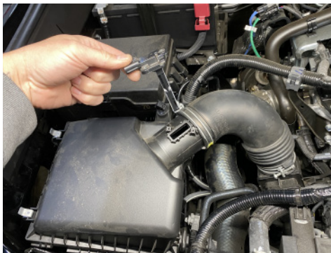
4. Unbolt MAF and remove from factory intake.
