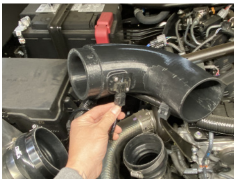
19. Reconnect the MAF sensor connector.
