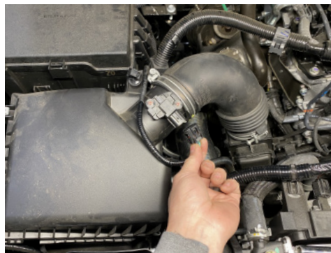
3. Disconnect MAF sensor connector.
