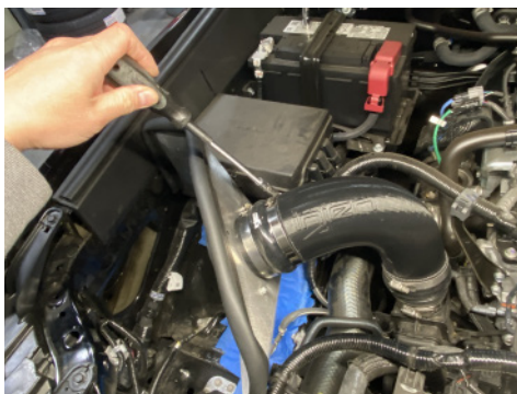
20. Install and secure intake tube.
