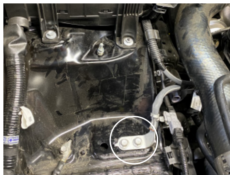
9. Locate factory chassis ground.
