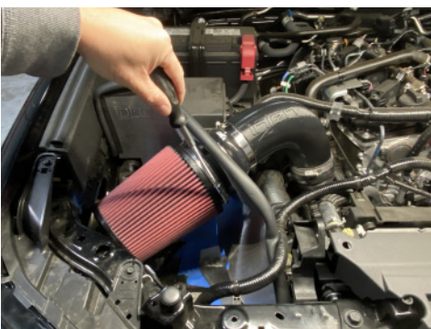
22. Install air filter and secure to assembly.
