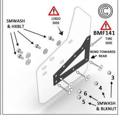
**IMAGE D/E** Place logo-side of flap facing rear bumper. Install SMWASH & 1.5SS6TR into mounts 1 & 2. 5SP mounts behind flap mount 2. Align flap to vehicle before tightening fasteners.
