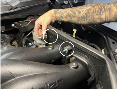
28. Install (2) two provided vibramounts onto heat shield. **Preinstalled bracket not shown.
