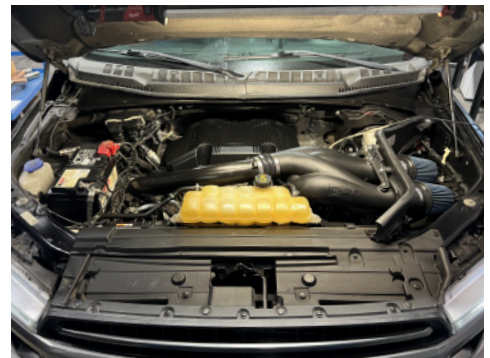
30. Install intake air temperature sensor into intake tube and secure.
