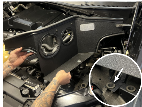
18. Position heat shield into vehicle making sure to align stand-off stud to factory mounting grommet.
