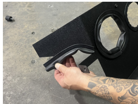
15. Install 7.5" rubber bulb trim (X-6058) to front lower portion of heat shield. Trim excess material as needed.
