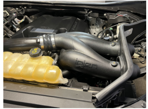
27. Secure intake tube to both driver and passenger side turbo inlet hoses.
