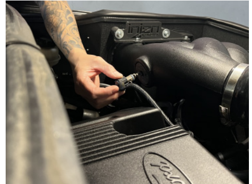
30. Install intake air temperature sensor into intake tube and secure.
