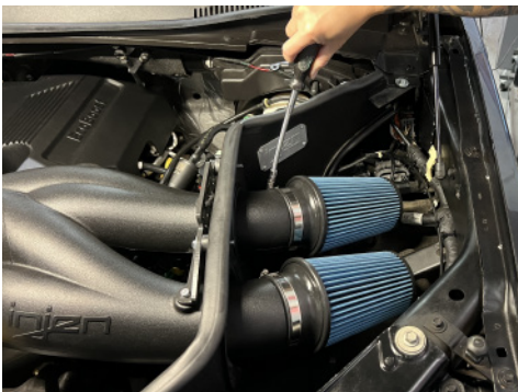
31. Install and secure both X-1079 air filters onto intake tube.
