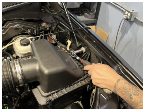
3. Unbolt 13mm bolt holding air box assembly to chassis.
