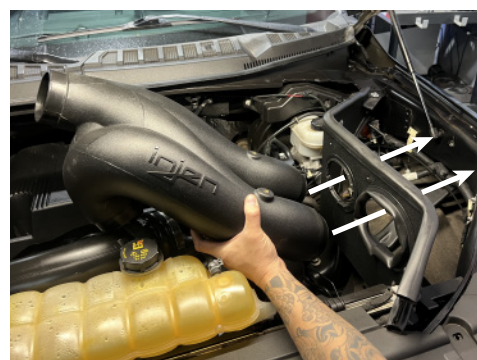
24. Carefully feed intake tube through heat shield.
