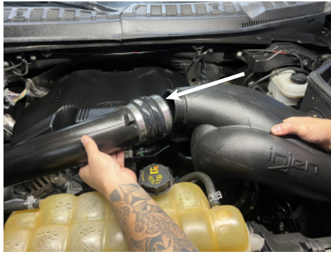
26. Insert upper outlet of intake tube into passenger side turbo inlet pipe.
