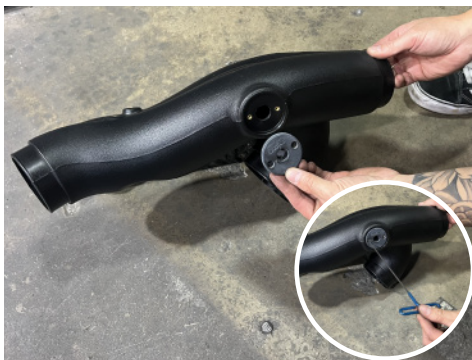
23. Install provided air temperature sensor adapter onto intake tube using provided button head screws.
