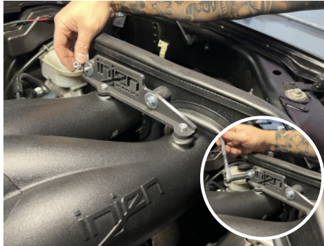
29. Install mounting bracket onto vibramounts on heat shield using provided hardware and secure.
