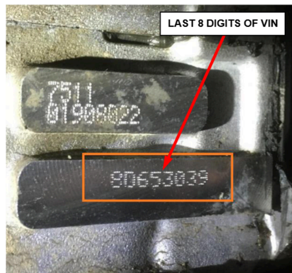
Figure 2 – Engine Identification Number
