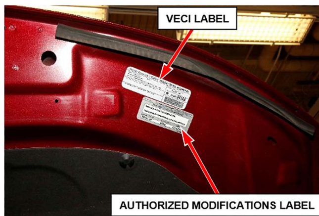
Figure 16 – Apply Authorized Modifications Label Near VECI Label (Specific Vehicle May Look Different)
