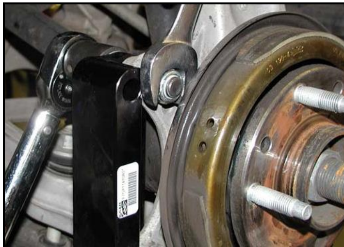
Figure 2: Installation of the intermediate bracket
