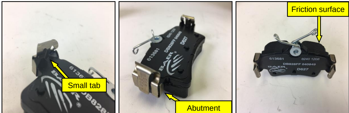
Figure 6: Pad abutment installation
