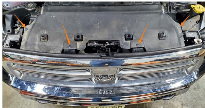
3. Remove the four (4) bolts securing the grille to the vehicle. Then, remove the grille from the vehicle by pulling it away from the vehicle to disengage the clips securing the bottom.
