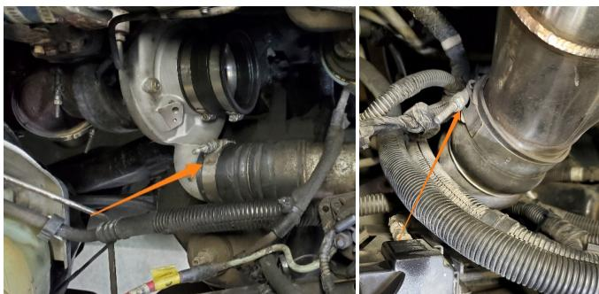
**13.** Install the Mishimoto boots and intercooler piping onto the vehicle with the supplied clamps, as shown below.
