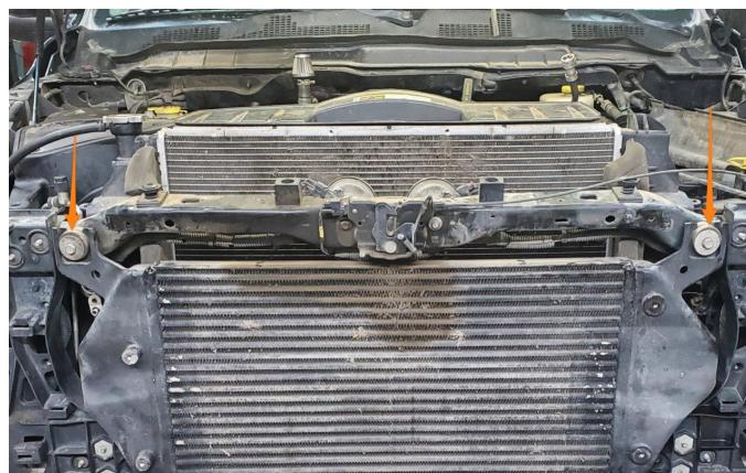
**11.** Transfer the rubber grommets from the stock intercooler to the Mishimoto intercooler and install the supplied metal shroud with the two (2) supplied M6 x 16mm bolts, as shown below. (Image on the next page)
