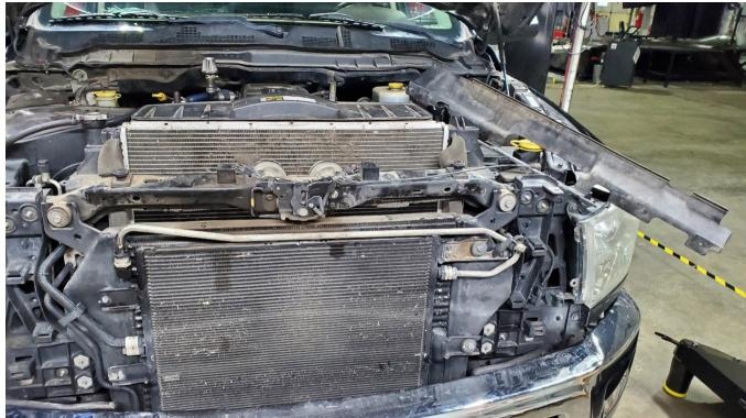
**5. BE SURE THE REFRIGERANT HAS BEEN PROPERLY RECOVERED BEFORE PERFORMING THIS STEP.** Remove the two (2) bolts securing the junction of the A/C condenser lines. Then, remove the one (1) bolt securing the junction to the intercooler.
