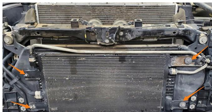
**9.** Remove the clamps that secure the intercooler pipe boots to each side of the intercooler.
