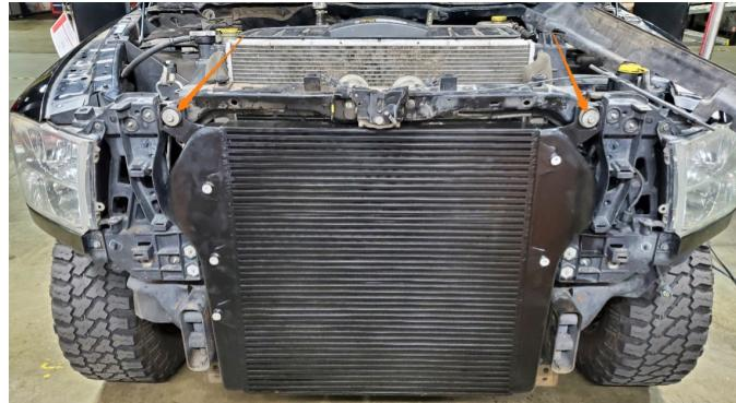
**15.** Reinstall the A/C condenser/transmission cooler and lines and secure them to the intercooler with the four (4) bolts that were removed in step 8.
