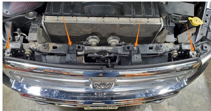
4. Remove the two (2) tree clips securing the shroud to the upper radiator support and slide it along the hood release cable to position it out of the way.
