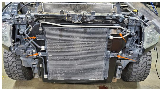
**16.** Reconnect the transmission cooler lines and reinstall the dust caps onto the fittings. Then, replace the seals at the A/C condenser line junction with new seals and reconnect the A/C condenser lines with the two (2) bolts removed in step 5. The bolt that mounted the junction to the stock intercooler will not be reused. [\(Image on the next page\)](#)
