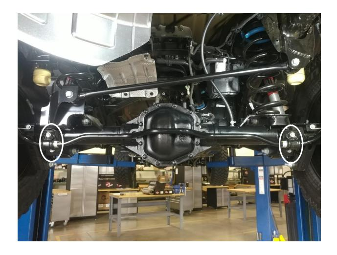
6. For Gladiator: Remove the four (4) bolts connecting the sway bar to the axle and move the sway bar out of the way.
