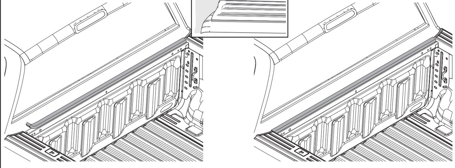
**4** Place the assembled bed cover (A) over the cab end of the truck bed. **NOTE:** Take care not to damage or deform the seals when installing the bed cover onto the truck bed. Visually check to ensure the front bed cover frame is even on both sides and square with the bed. Make sure the cover is centered on the bed of the vehicle before tightening clamps.
