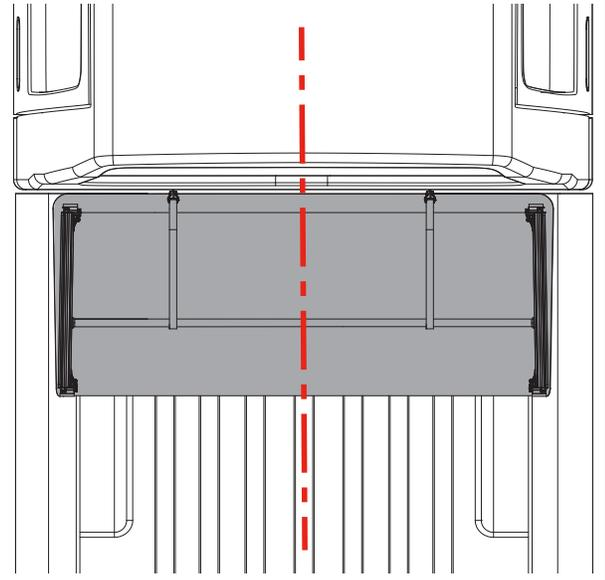
**5** Unfold the bed cover fully and adjust the position over the truck bed for proper cab and tail alignment. Then carefully refold the bed cover without shifting its position on the truck bed. **NOTE:** Ensure the tail seal contacts the tailgate cap as shown.
