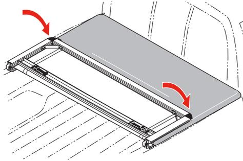
**!** **IMPORTANT:** Before folding the second section of the cover, the rear clamps must be stowed into the rail to prevent damage to the fabric. Failure to stow the handles will puncture the tarp and void the warranty.
