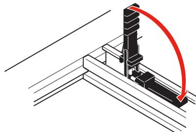
**!** Fold the cover forward and fasten the straps in the middle section to the front rail. Failure to do so could allow the wind to blow the cover back resulting in damage to the cover and truck. Check that the straps are tight.
