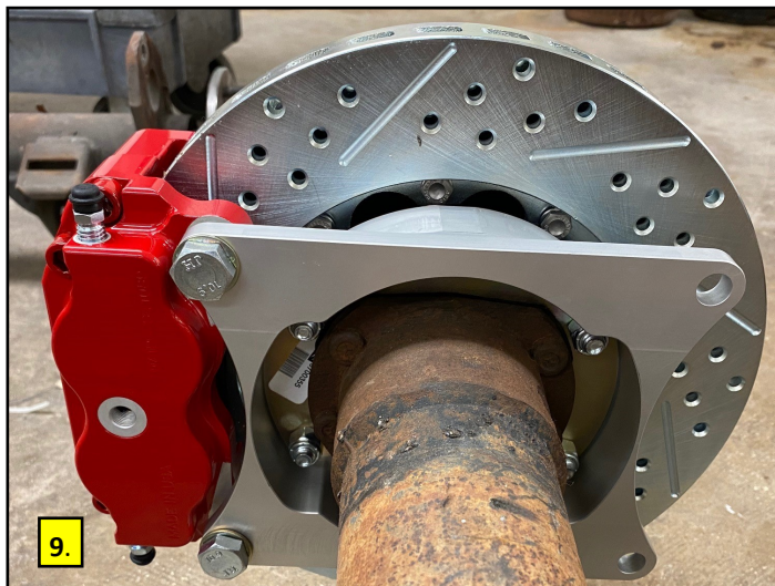
9. Inboard view of the installed bracket, rotor and caliper.
