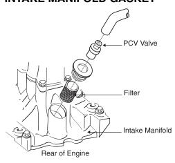
**IMPORTANT:** 1986 and later Ford 5.0L applications, require the replacement of the crankcase breather filter, located under the PCV Valve. If the filter is not replaced the filter can get clogged with the carbon and sludge resulting in increased crankcase pressure, intake manifold end seal leakage, timing cover or rear main seal leakage.
