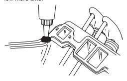
**PRIOR TO REINSTALLING INTAKE MANI-FOLD** apply a small dab of silicone sealer, to the 4 corner intersections between the end seals and gaskets.
