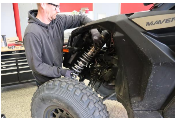
Step 17. Install shock in vehicle in reverse of removal.
