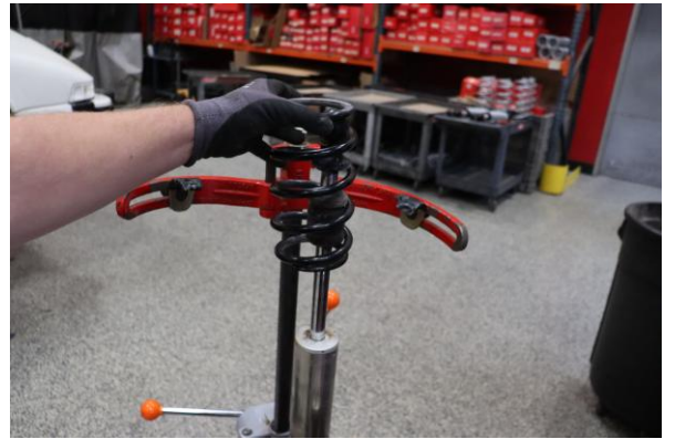
Step 10. Remove OE front secondary spring.
