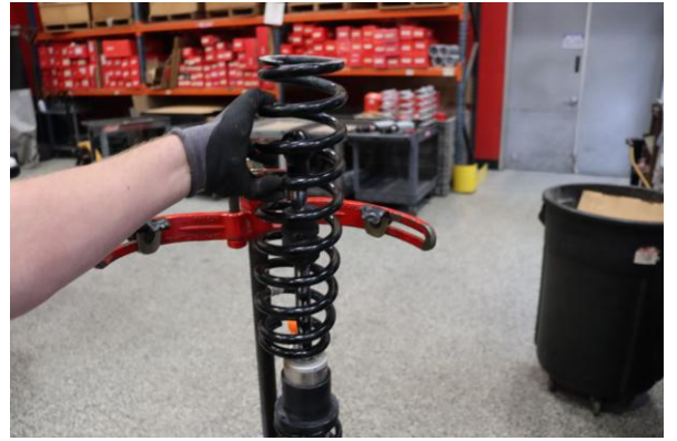
Step 8. Remove OE front main spring.
