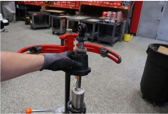
Step 9. Remove OE slider.
