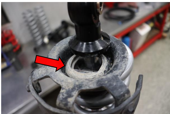
Step 17. OE rear lower spring seat has a flat cut on both rod end and seat. Make sure they are seated together.
