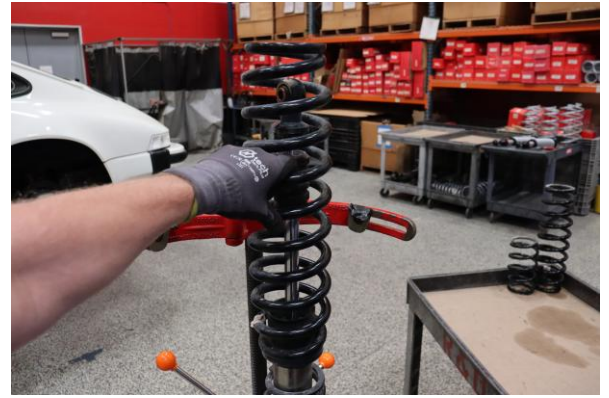
Step 8. Remove OE main spring.
