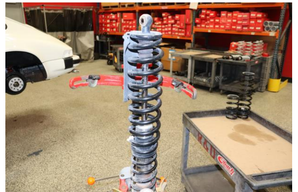
Step 6. Use a spring compressor to compress spring assembly.
