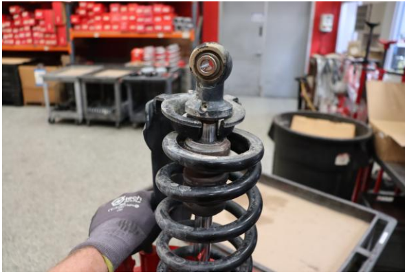
Step 7. Remove lower spring retainer and decompress the spring
