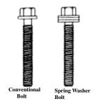
The gasket(s) included in this set will function with manifolds having either "Conventional" or "Spring Washer" style bolts.
