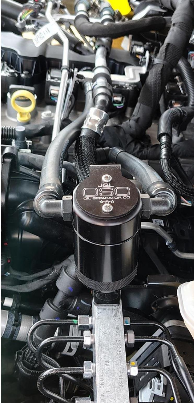
8 Check oil separator after 1000 miles of driving to gauge how often it needs to be emptied. Every vehicle is different!
