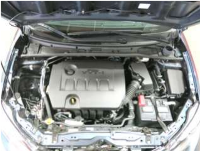
STOCK INTAKE INSTALLED
