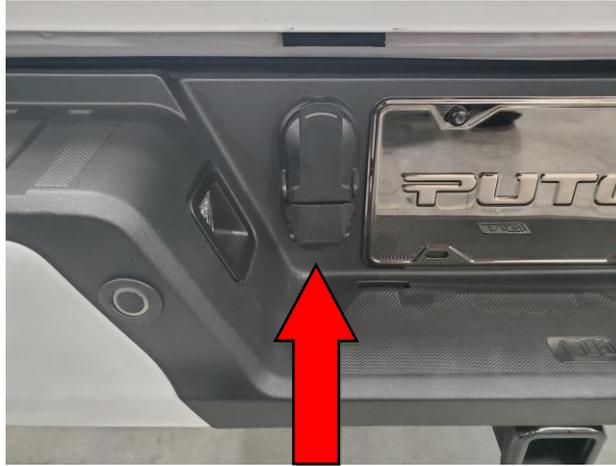
2. Plug the other end of the Quick Connect Harness into the 7-pin plug on the bumper. **Refer to Figure 3.**
