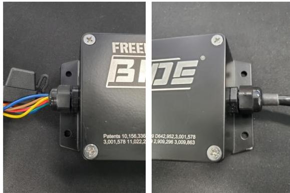
The Freedom Blade driver box comes with two predrilled holes on a flange on each side of the driver box. This allows the driver box to be mounted in many different orientations and places behind the bumper of your truck. Try to use at least three of the four mounting holes to secure the driver box.
