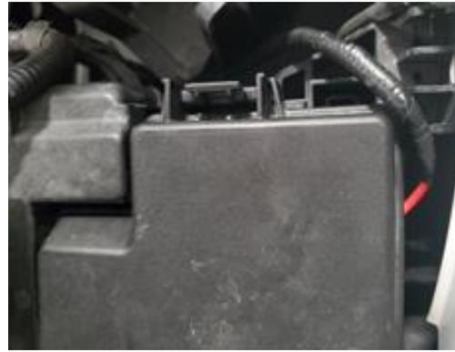
4. Carefully fish #5, the long bundle of wire with a spade connector down through the engine bay and away from any components that get hot or move such as the engine block and exhaust.
