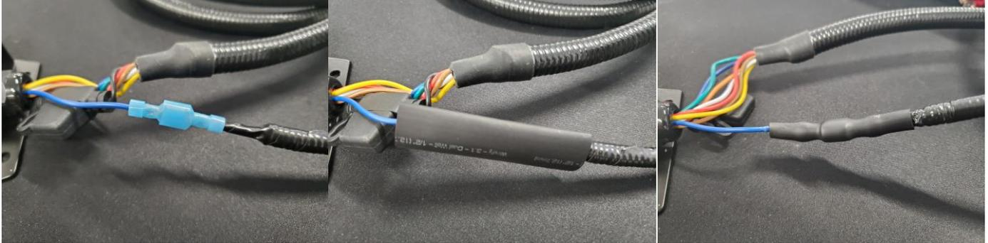
1. The power wire connects to the freedom blade using a spade terminal. Once connected, slide the supplied heat shrink over the connection and use a heat gun or lighter to shrink the heat shrink onto the connector. This heat shrink has adhesive on the inside which will create a permanent, water tight seal.
