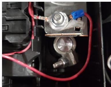
2. Attach the #4 (red wire) with a 3/8" ring terminal to the battery positive terminal.
