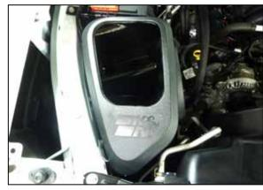
11. Install the K&N air filter housing into the vehicle so the mounting posts insert into the factory mounting grommets. Secure the air box with the factory nut from the previous step.
