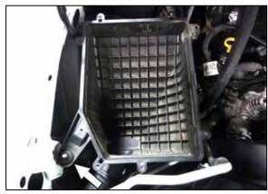
7. Remove the nut that secures the lower air filter housing and then lift the lower housing up to dislodge it from the mounting grommets and remove it from the vehicle. NOTE: The nut will be reused in the next step.
