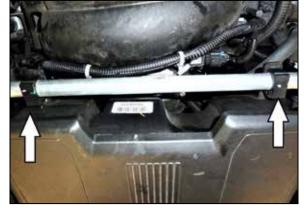
2. Separate the coolant pipe from the rear of the intake plenum by disconnecting the retaining clips from the plenum.
