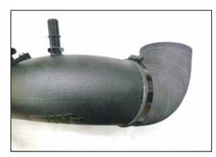
17. Install the elbow coupler onto the K&N intake tube as shown but do not fully tighten the hose clamp.
