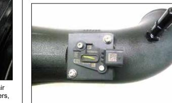
16. Install the mass air sensor assembly onto the intake tube using the provided hardware as shown. The sensor should be positioned as shown in the photo.
