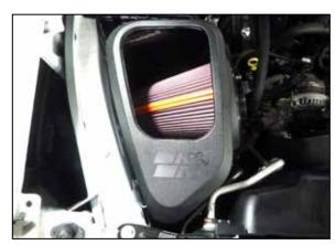
13. Install the K&N air filter into the K&N air filter housing.
