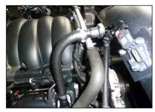
21. Install the CCV hose assembly onto the valve cover port and quick connect fitting installed into the K&N intake tube.
