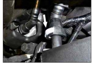
3. Push in the locking tabs on the CCV quick connect fittings and then remove the CCV hose assembly from the vehicle.
