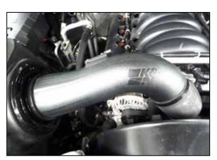
18. Install the K&N intake tube assembly into the K&N air filter and then connect the coupler to the throttle body, adjust the tube for best fit and then secure with the provided hose clamps.
