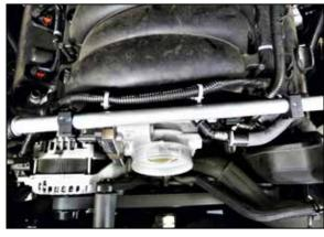
10. Secure the wiring harness and coolant pipe to the bracket as shown.
