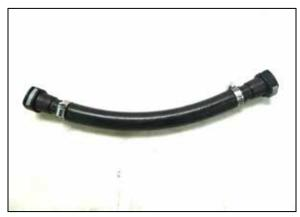
20. Assemble the provided CCV hose and quick connect couplers with the provided hose clamps.
