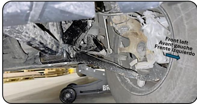
**Step 1:** Raise vehicle safely, turn wheels left to install left kit, right to install right kit, and install from front.
