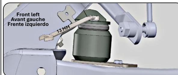
**Step 7:** Mount spacer (#11) and Aeon Spring (#10) with washer (#9) and bolt (#12) using 13mm wrench.
