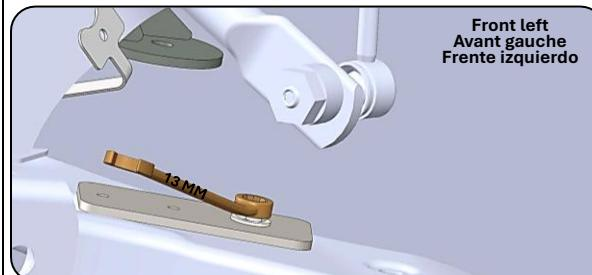
**Step 6:** Place item (#5) on control arm, align holes and make edge face parallel to bracket (#1). Drop bolt (#8) with washer (#9) into hole, through disc (#6), tighten with item (#7) to secure.
