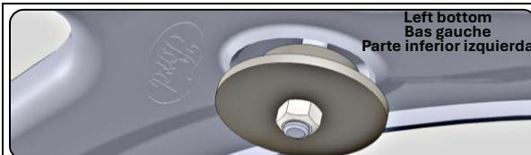
**Step 5:** Align item (#6 & #7) under control arm hole and hold.
