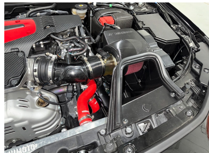
Figure 3: 3D printed Mishimoto intake prototype
