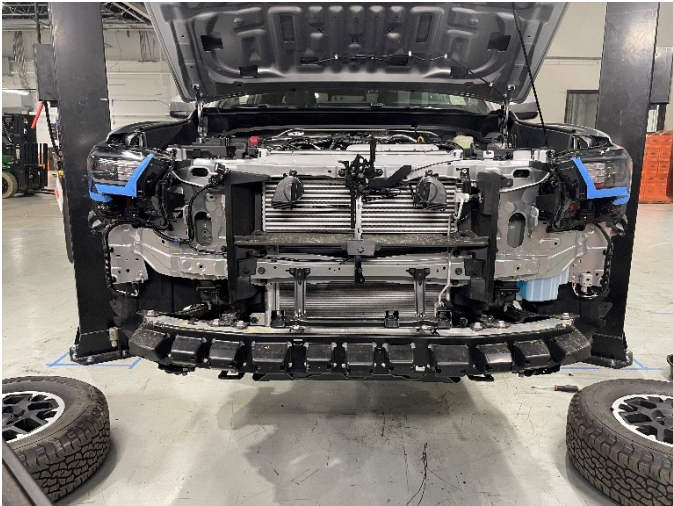
Figure 1: 2024 Toyota Tacoma with the front bumper cover removed, showing the factory intercooler and ducting.
