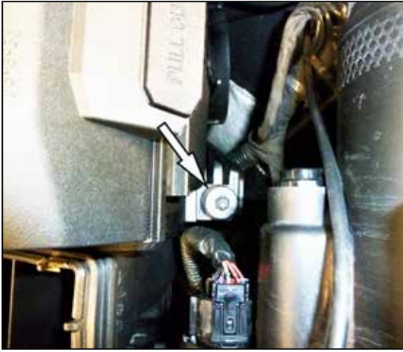
7. Remove the front air filter housing mounting bolt shown.
