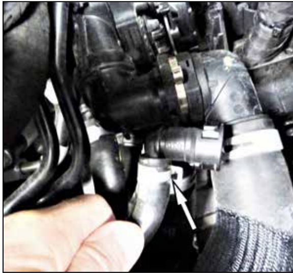
13. Release the spring clamp that secure the 90degree quick connect fitting from step #5 and then remove the fitting and replace it with the straight quick disconnect fitting provided.
