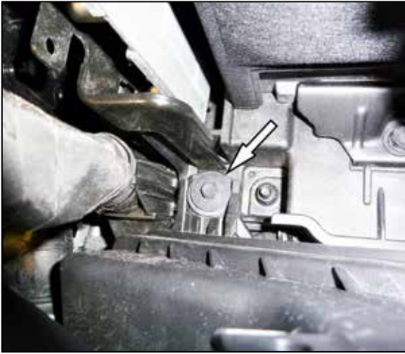
8. Remove the rear air filter housing mounting bolt and then remove the air filter housing from the vehicle. NOTE: K&N Engineering, Inc., recommends that customers do not discard factory air intake.
