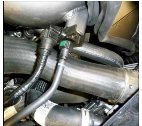
18. Reconnect the Ejector fitting vent line connections.
