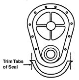
ATTACH AND ALIGN GASKET: Apply a quick-drying adhesive sparingly in several places on the engine casting or block. Attach gasket(s) on surface where adhesive was applied. Allow time for adhesive to set. Test for slippage with light pressure. If gasket moves, allow more time.
