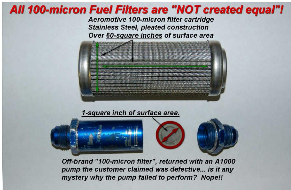
You may run any brand of filter you choose on your car, just be certain that it meets the following requirements: *The filter element used on the inlet side of any Aeromotive fuel pump may be no finer than 100-micron (no number smaller than 100), with a surface area of 60 square inches or more.*
