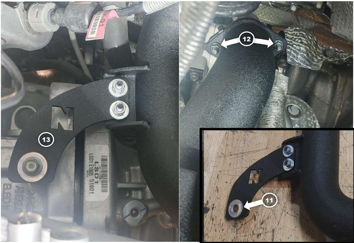
14. Loosely install the supplied bracket to the upper hot side charge pipe as shown using the two (2) M6 Flat Washers and two (2) M6 Nylon Lock Nuts included.
