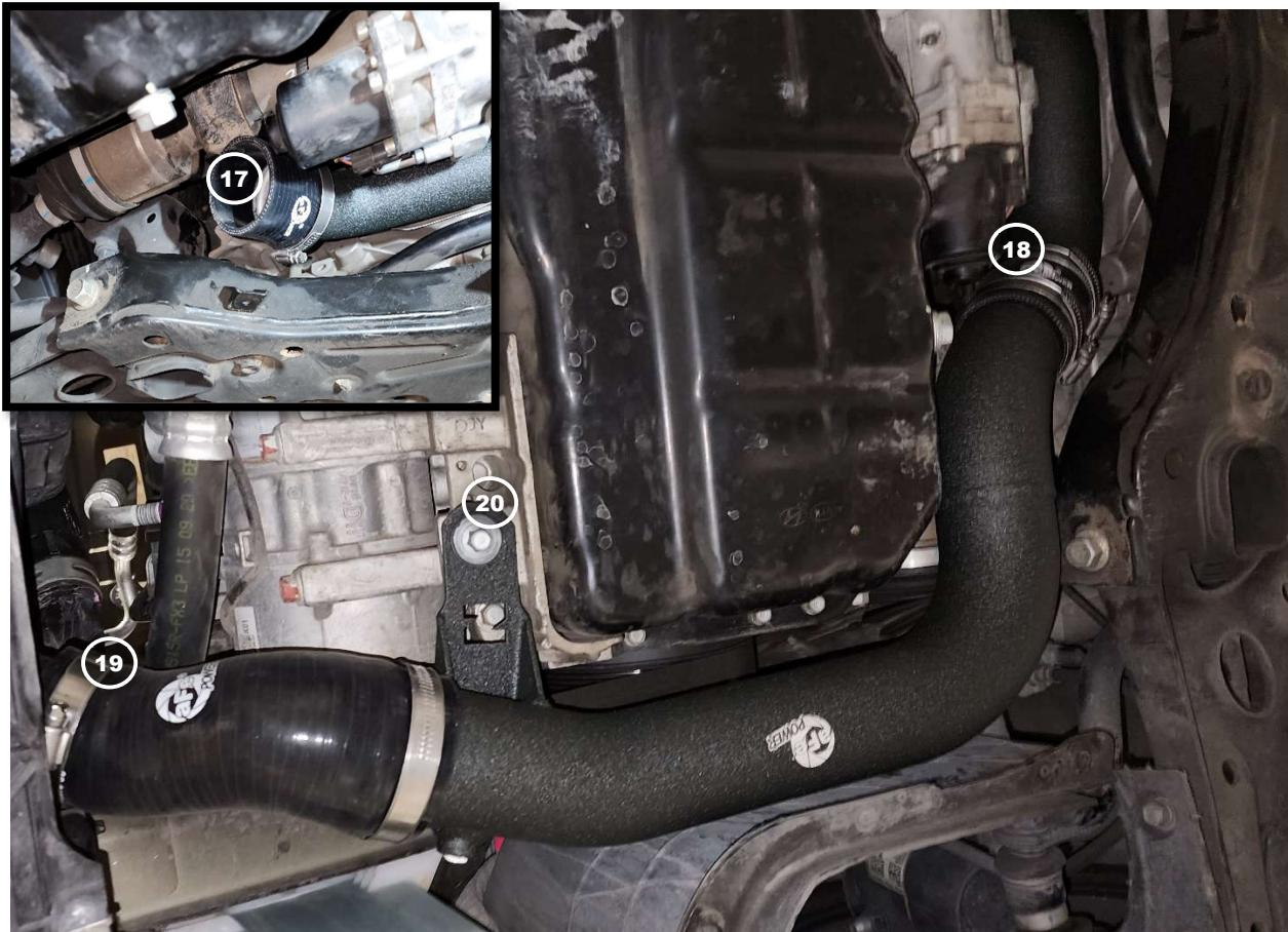
**Note: Be sure to thoroughly clean all oil residue off of the connections before installing any of the aFe charge pipes into the vehicle**
