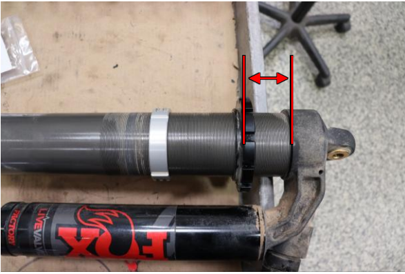
Step 13. Set pre-load to 50mm (2") from bottom of spring seat to bottom of reservoir bridge collar.
