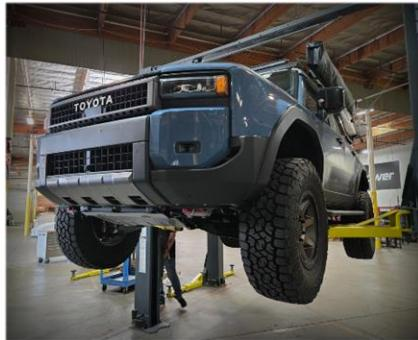
2. Remove the factory skid plate by removing the (4) bolts in green and loosen the (2) bolts in red. The skid plate should slide to the passenger side and drop.
