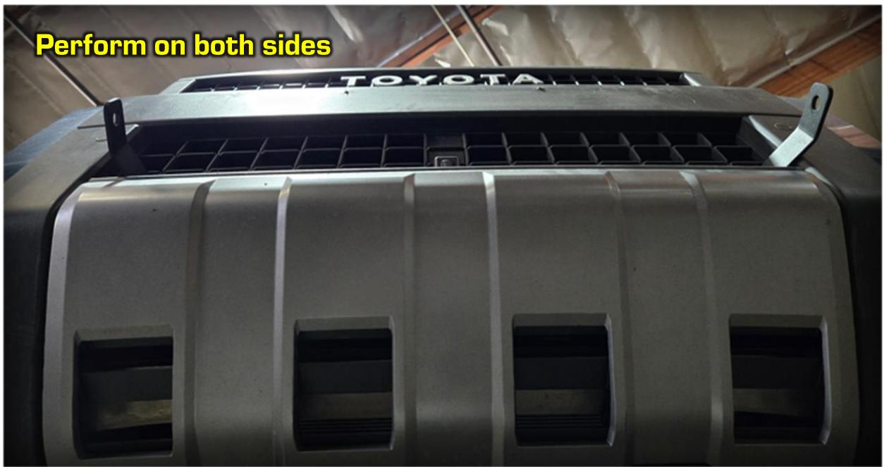
6. Next, unbolt the (2) bolts holding each of the factory tow hooks. Remove on both sides. Factory tow hooks will not be re-installed but keep hardware.
