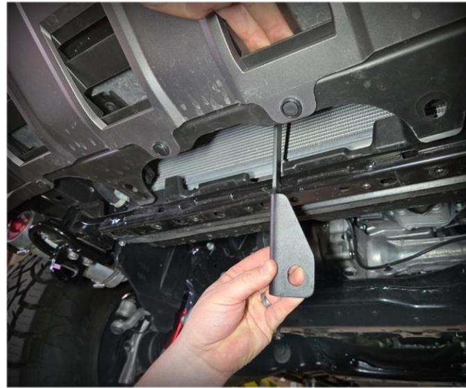
Bracket should pop out of the bottom outer grill hole. Use the factory bumper beam bolt to fasten the bracket to the bumper beam but do not fully tighten yet.
