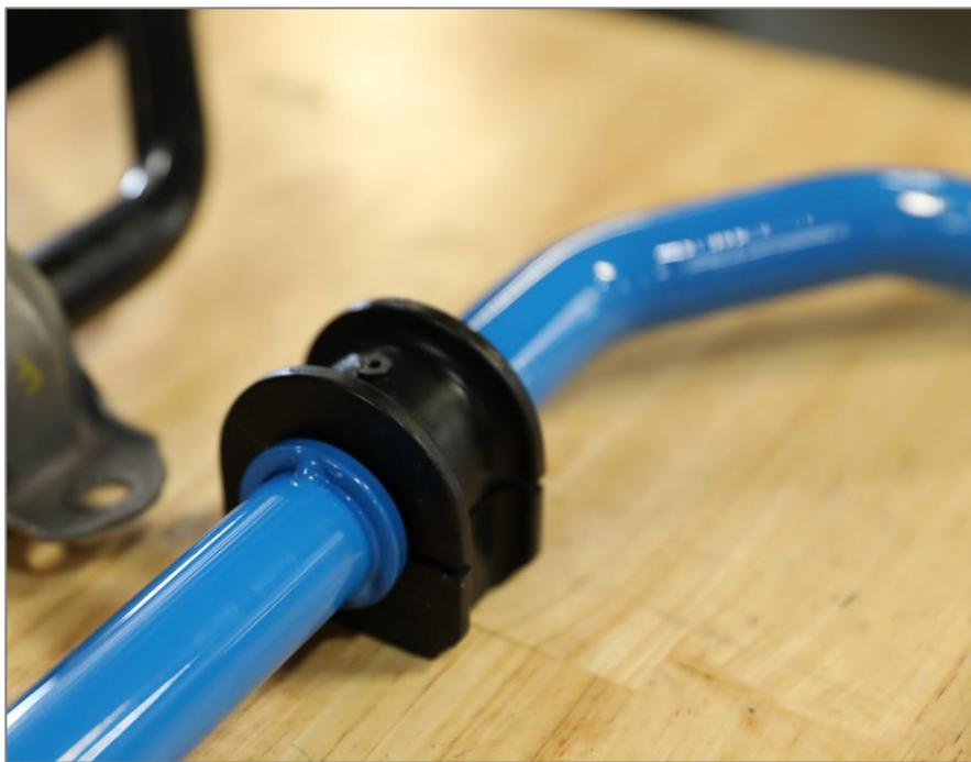
9F Install the front aFe Control sway bar in the same manner as factory removal. Place the factory base plate up to the subframe studs. Slide the aFe Control bushing bracket onto the bushings and mate the sway bar assembly to the subframe. Reuse the factory nuts to secure the brackets to the subframe. Fully tighten this hardware to **15 ft·lbs**.
