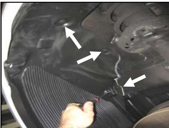
I. Remove the three upper clips on the fender liner.
