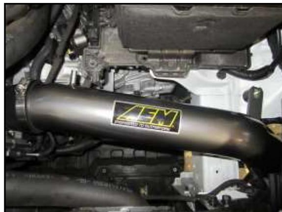
D. Install the AEM intake tube (C).
