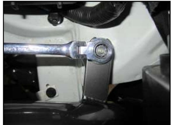
H. Make sure you have clearance around the filter and tighten the 6MM nut installed in step E.
