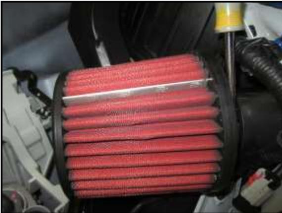
G. Rotate the AEM filter to allow for proper clearance and tighten the hose clamp on the filter.
