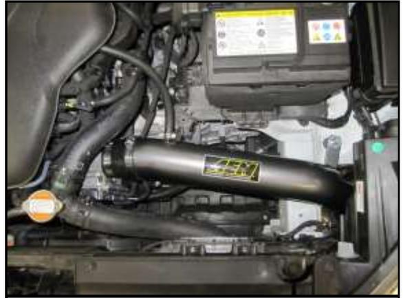
L. Check the fitment of the intake system and ensure there is clearance between the inlet pipe and its surrounding components. Once proper fitment is achieved check all the hose clamps and M6 nut on the rubber mount.
