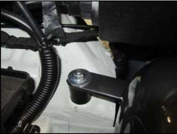
E. Install the 6MM washer (I) and nut (H) on the rubber mount.
